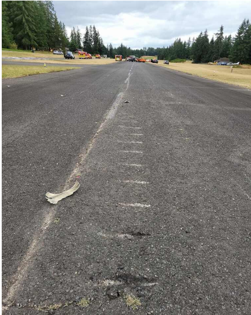
Figure 2: View of airplane's propeller contact marks leading down the runway. (Courtesy of Law Enforcement)
