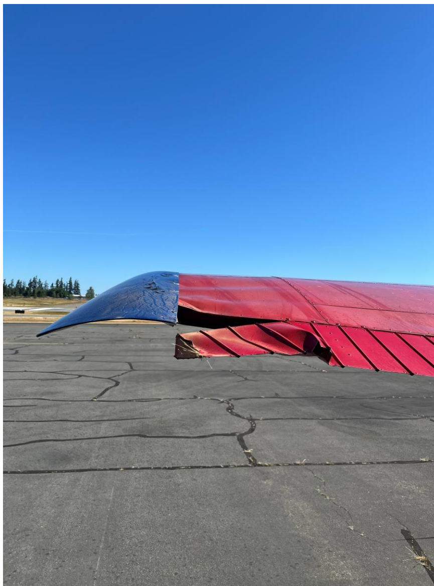
Photograph 3 - View of left aileron damage (Courtesy of Airport Operations)
