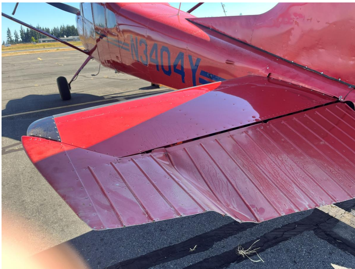
Photograph 2 - View of left elevator damage (Courtesy of Airport Operations)
