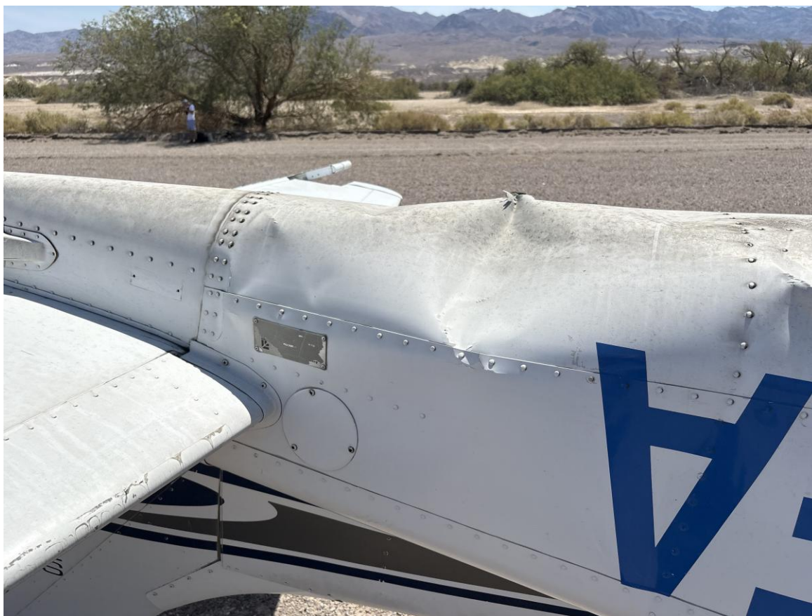
Photograph 3 - View of aft fuselage damage (Courtesy of National Park Service)
