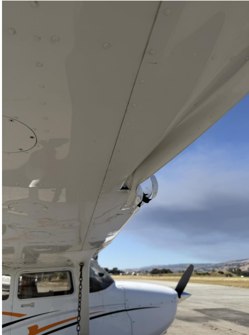
Photograph 3 - View of right wing damage (Courtesy of Pilot)
