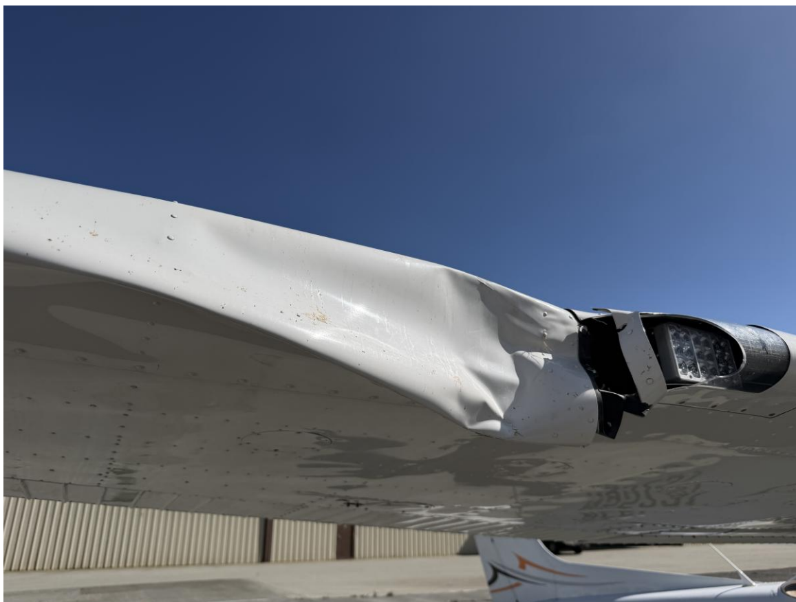
Photograph 2 - View of right wing damage (Courtesy of Pilot)
