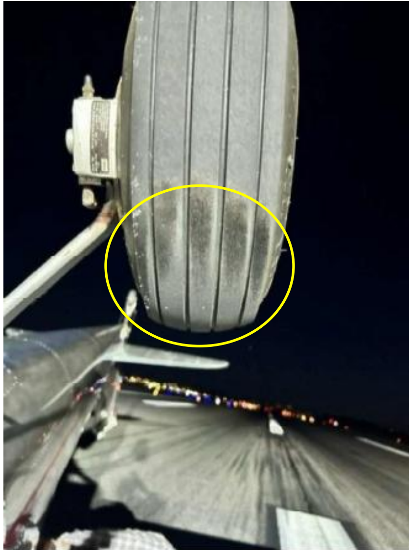
Photograph 4 - View of right main landing gear tire wear marks (Courtesy of Airport Operations)
