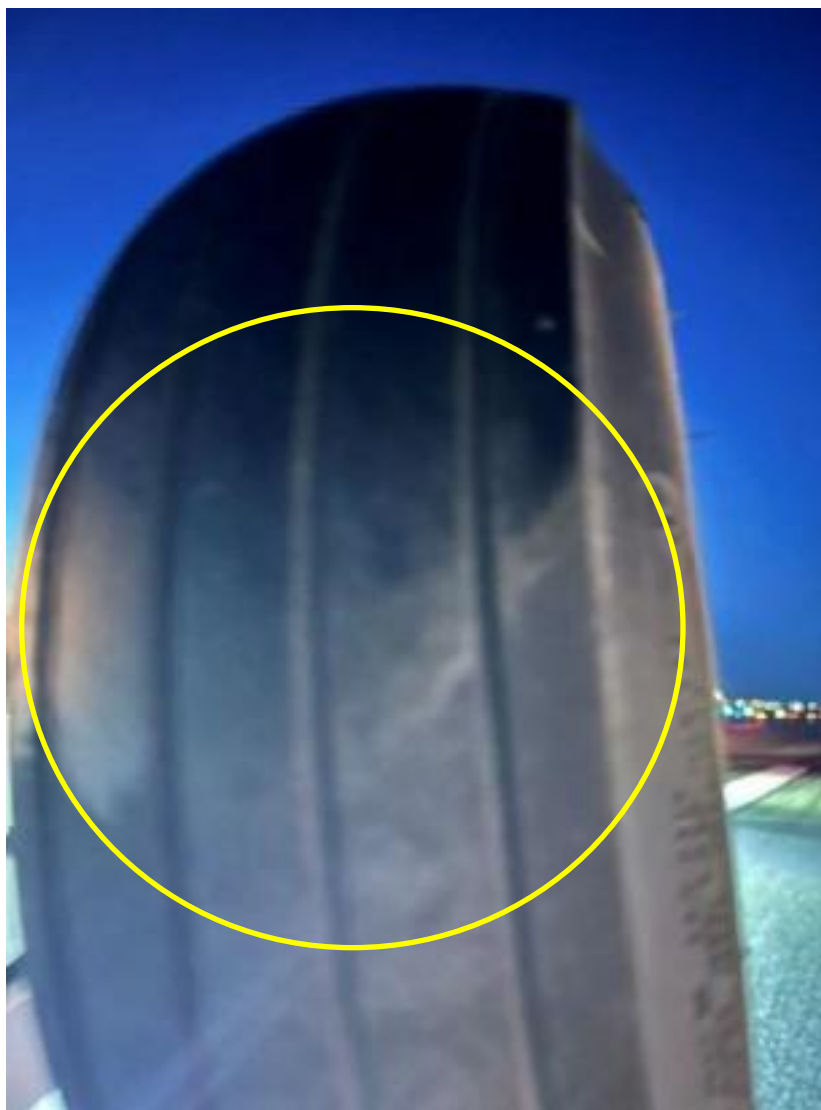
Photograph 5 - View of left main landing gear tire wear marks (Courtesy of Airport Operations)
