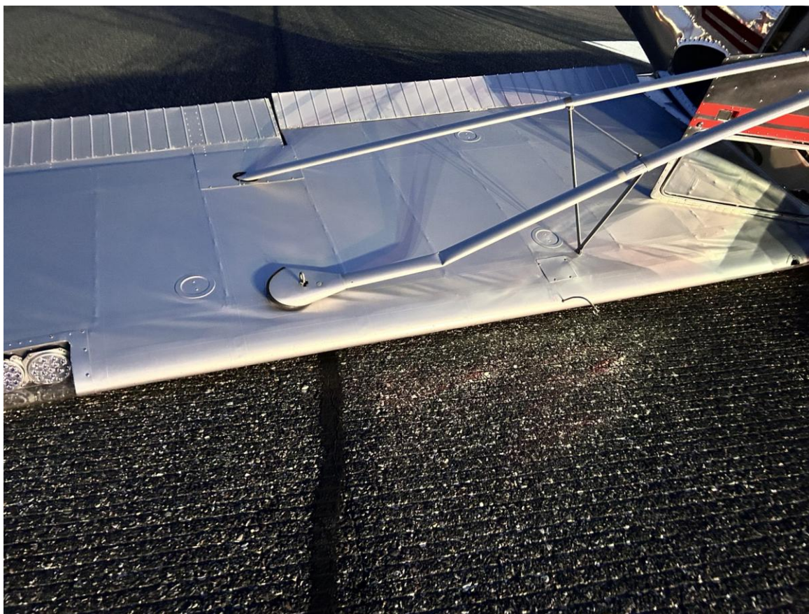
Photograph 3 - View of left wing lift strut damage (Courtesy of Airport Operations)
