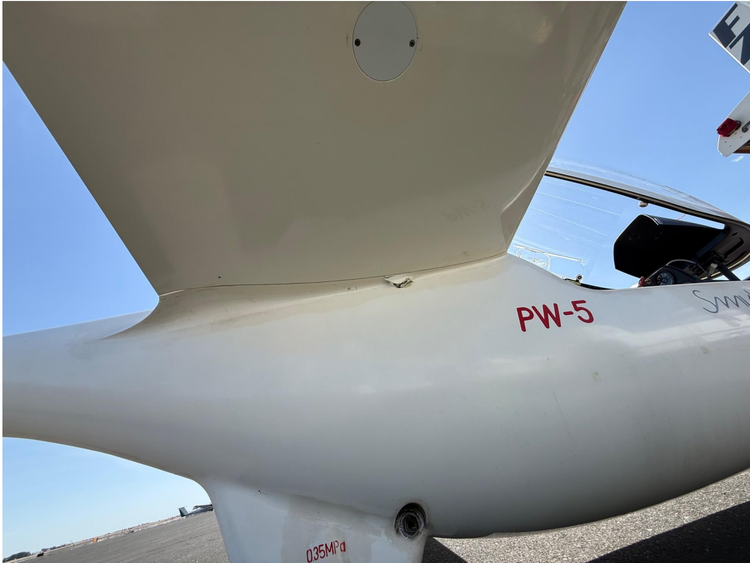
Photograph 3 - View of puncture under right wing. (Courtesy of Pilot)
