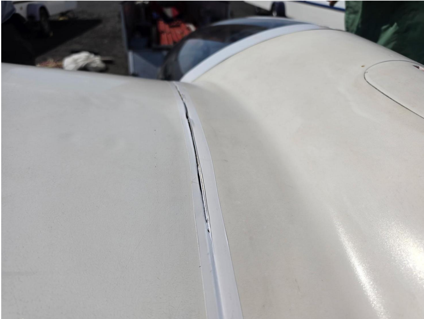
Photograph 1 - View of top left wing broken tape. (Courtesy of Pilot)
