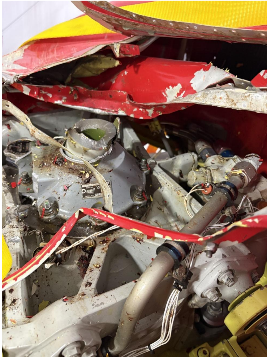
Photograph 4 - View of mast separation point.
