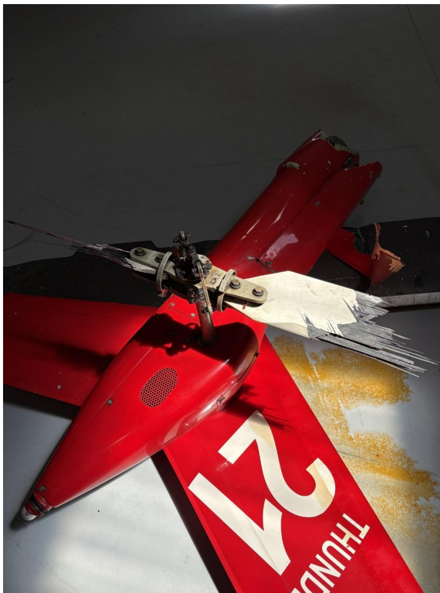
Photograph 2 - View of tail rotor and tailboom damage.
