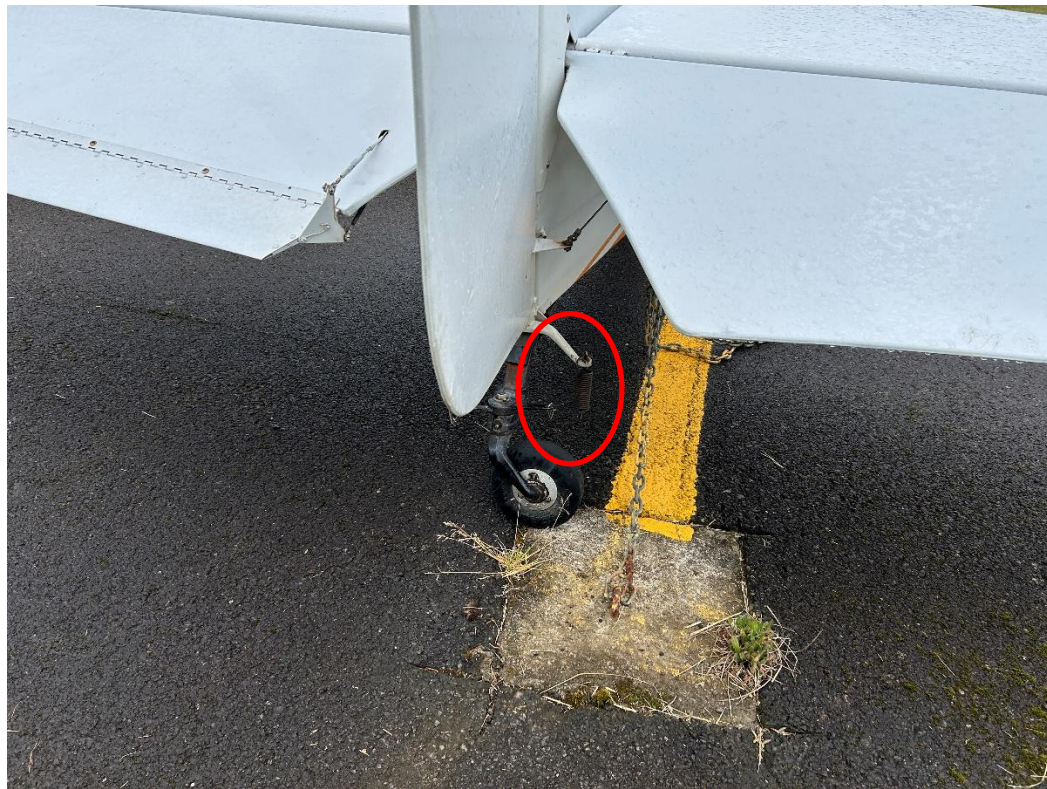
Figure 2: View of right tailwheel spring disconnected. (photo provided by the FAA)
