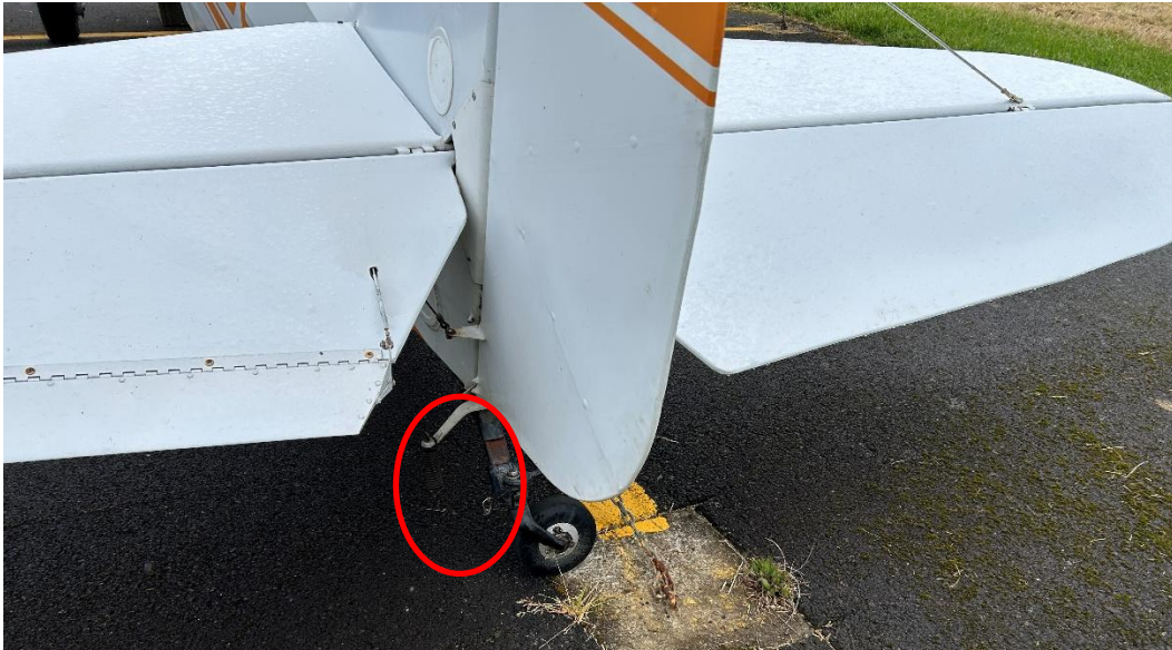
Figure 1: View of left tailwheel spring disconnected. (photo provided by the FAA)
