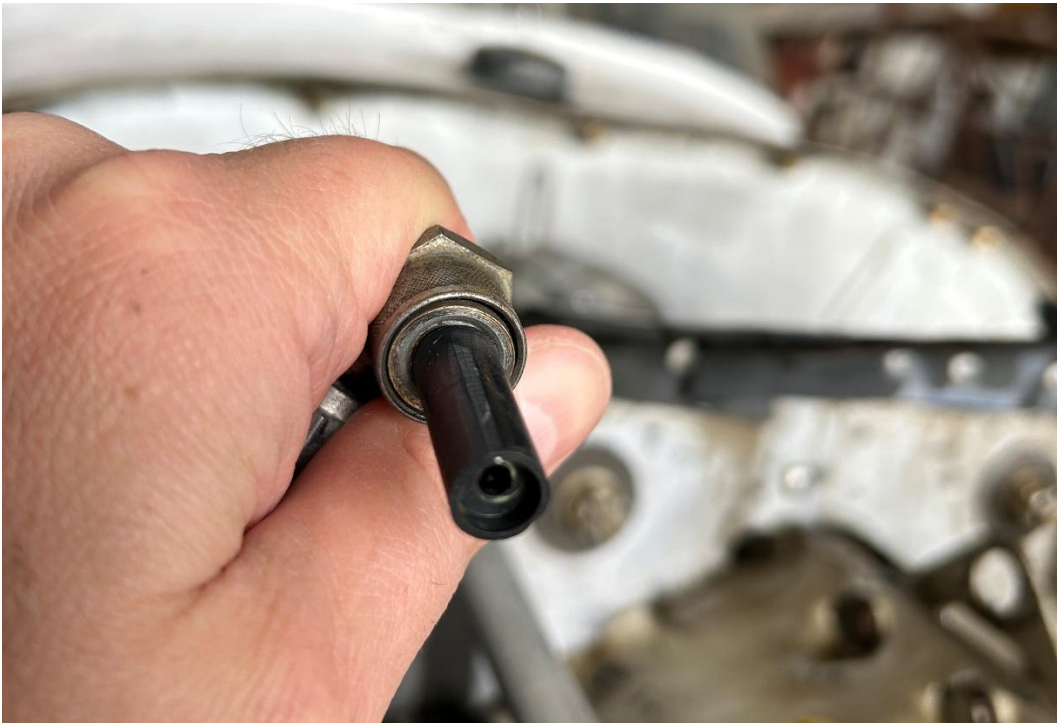
Figure 2: View of number 3 cylinder ignition lead conductor separation (photo provided by the FAA)
