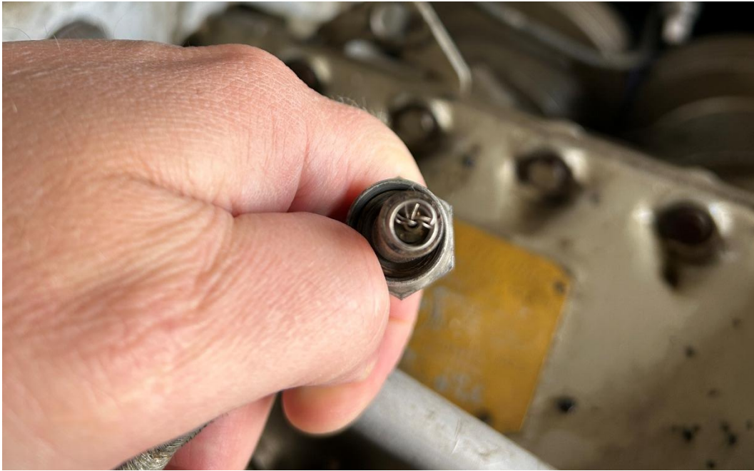
Figure 1: View of number 3 cylinder frayed ignition lead (photo provided by the FAA)
