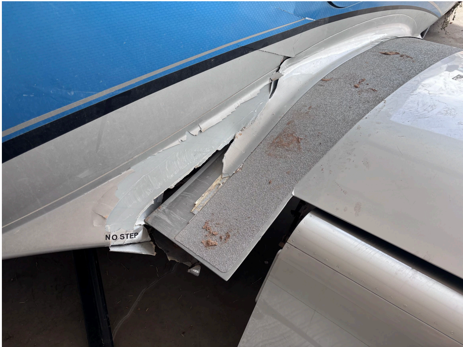
Photograph 2 - Top view of broken wing root (Courtesy of insurance company)
