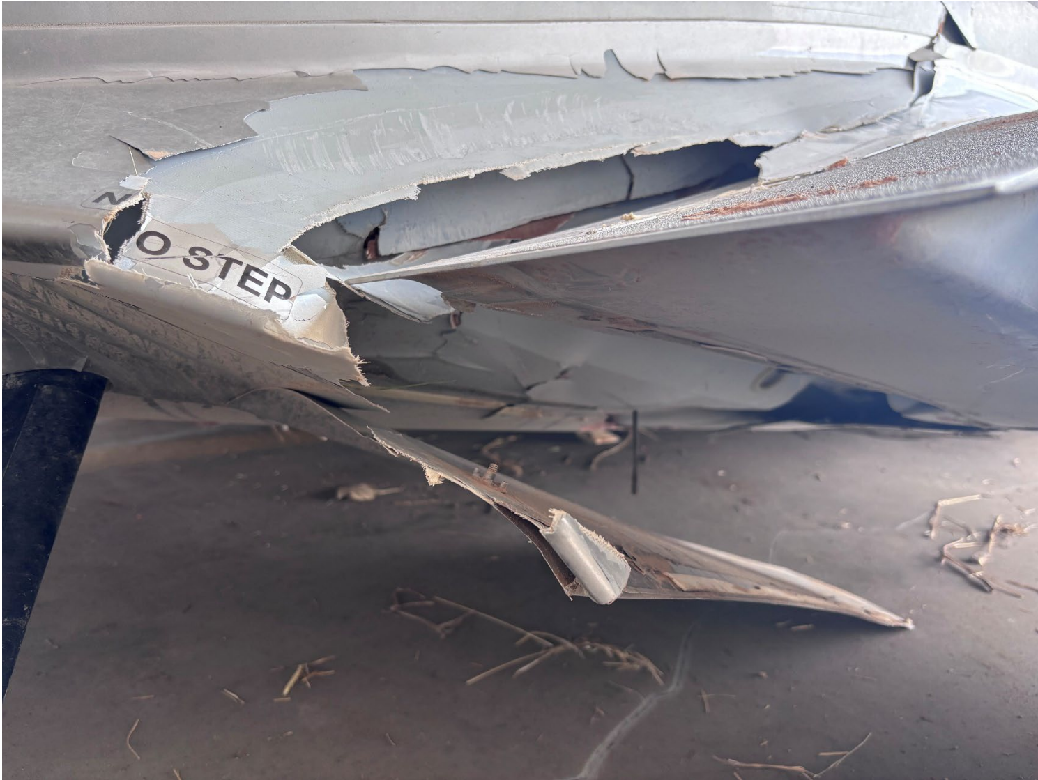
Photograph 3 - Underside view of broken wing root (Courtesy of insurance company)
