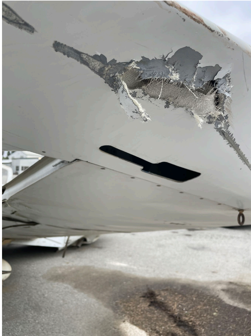
Photograph 2 - Damage, right wingtip (Courtesy of FAA)
