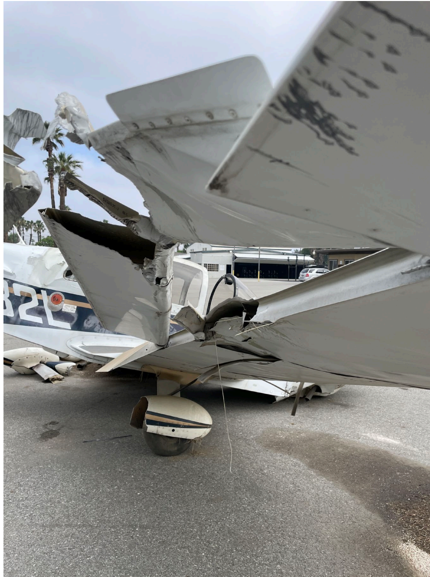
Photograph 3 - Damage, right wing (Courtesy of FAA)
