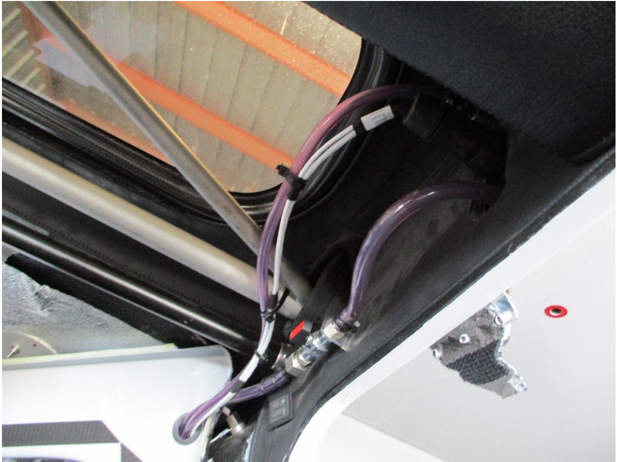
Photograph 4- View of fuel lines in the cockpit (Courtesy of Federal Aviation Administration)
