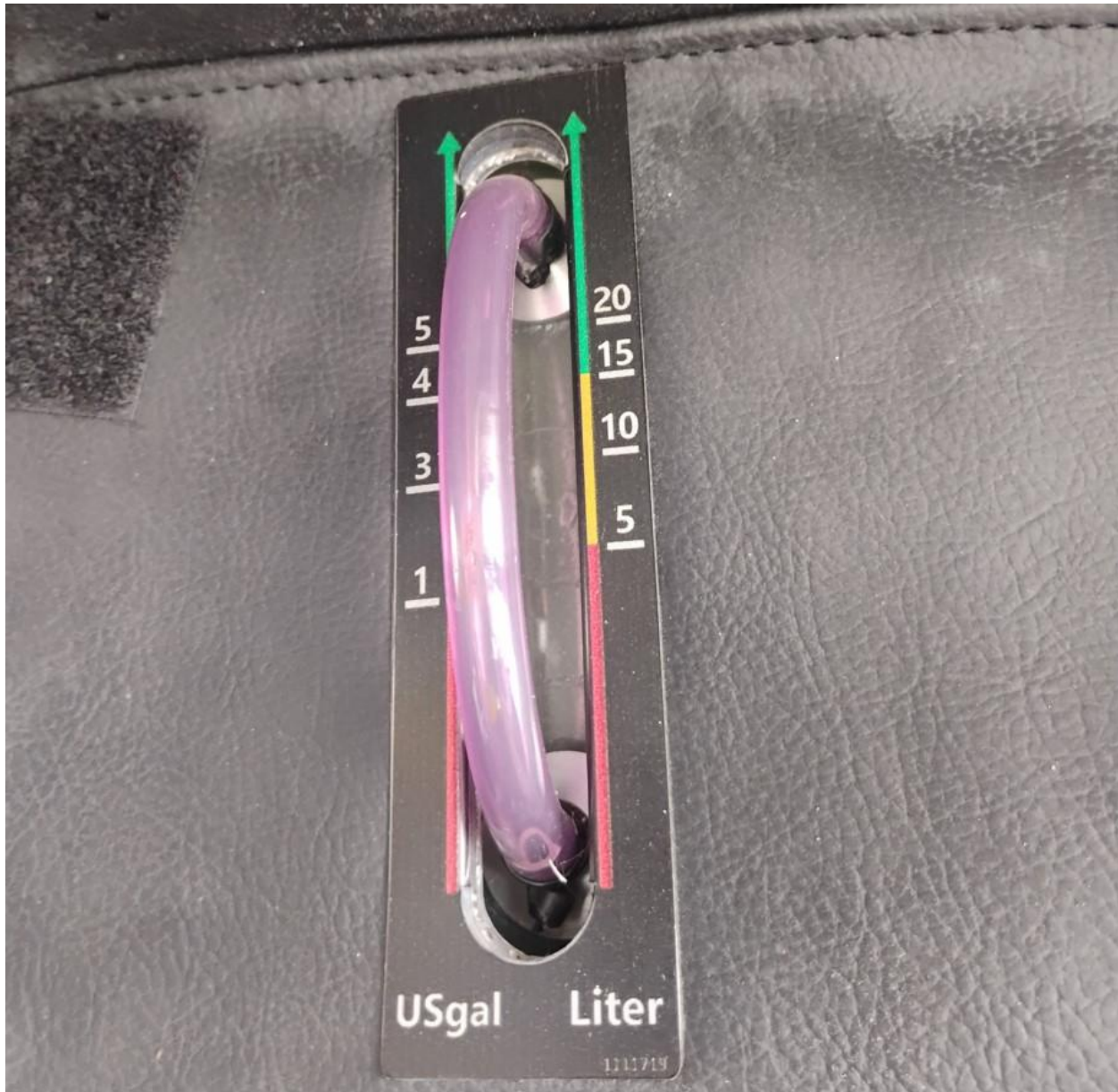
Photograph 2- View of left fuel sight gauge (Courtesy of Federal Aviation Administration)
