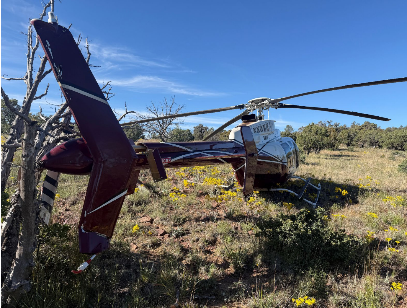
Photograph 2 - View from the left rear of the helicopter showing the tree and damage to the vertical stabilizer (Courtesy of pilot)
