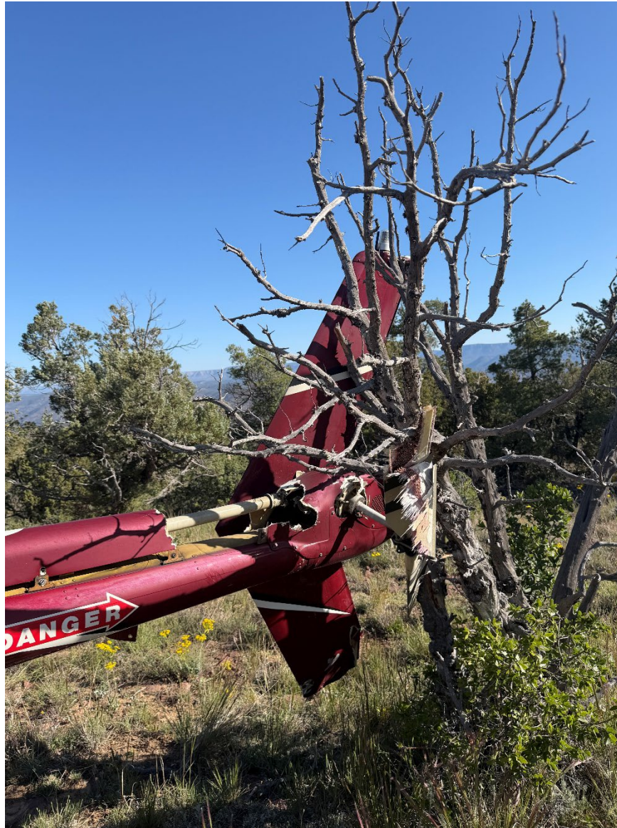
Photograph 3 - View of damage to vertical stabilizer and tail rotor (Courtesy of Pilot)
