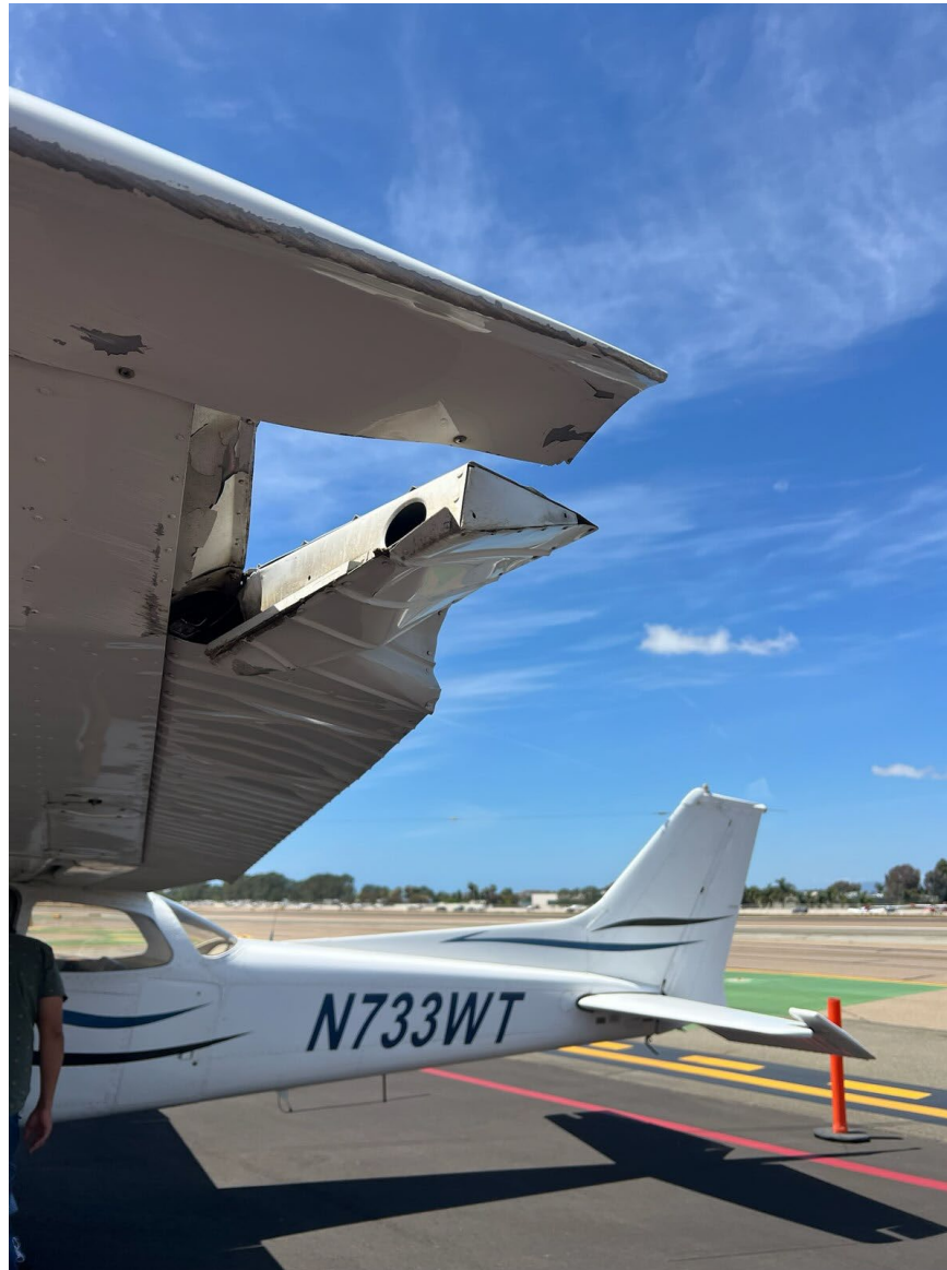
Photograph 2 - Rear View of Damaged Wing (Courtesy of Airport)
