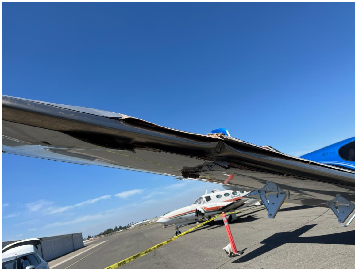
Photograph 2 - View of right wing damage (Courtesy of Federal Aviation Administration)
