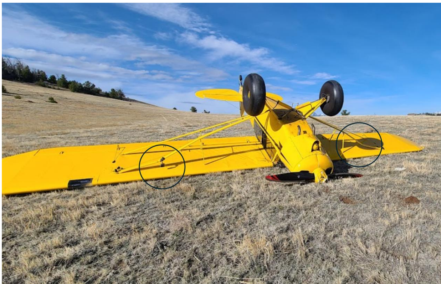
Photograph 1 - View of bent struts. (Courtesy of Pilot)
