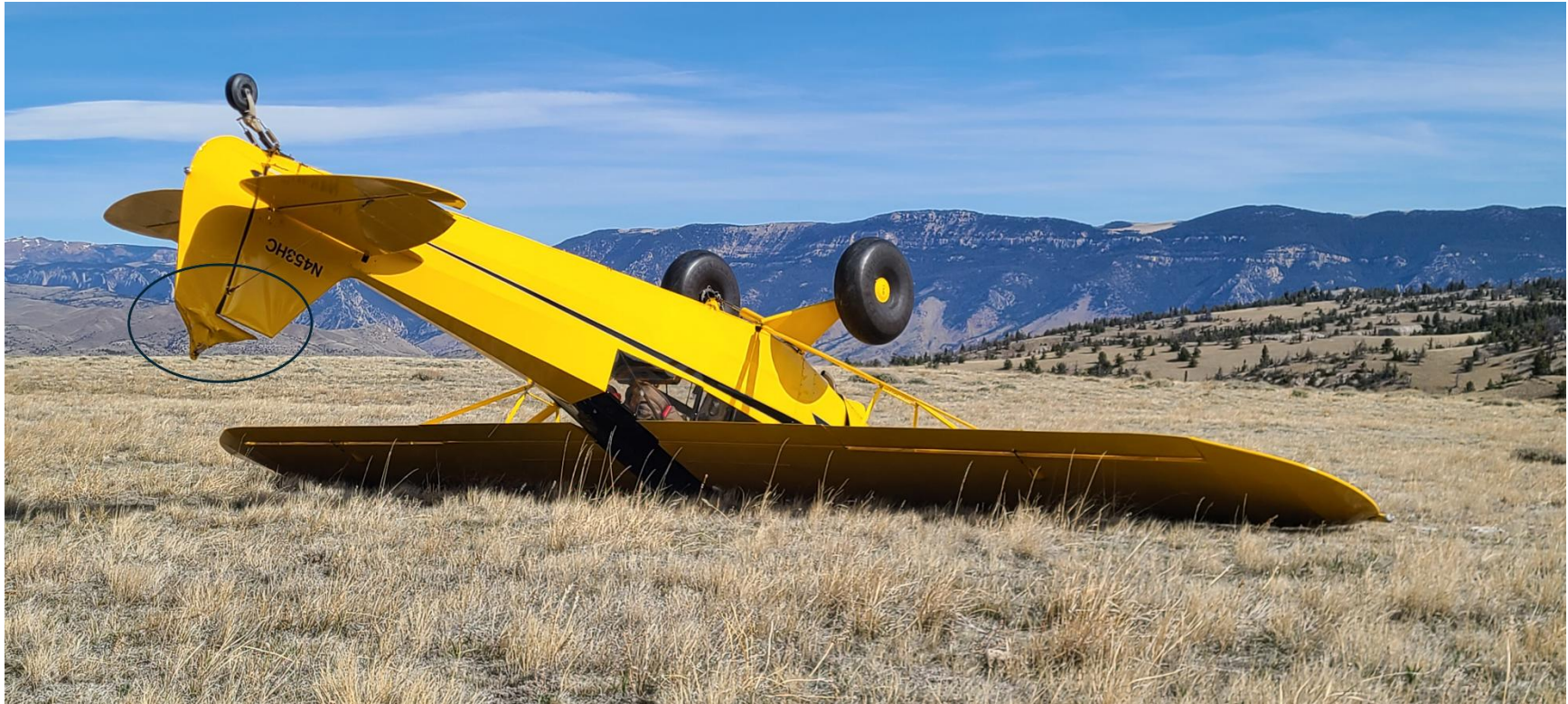
Photograph 2 - View of rudder damage. (Courtesy of Pilot)
