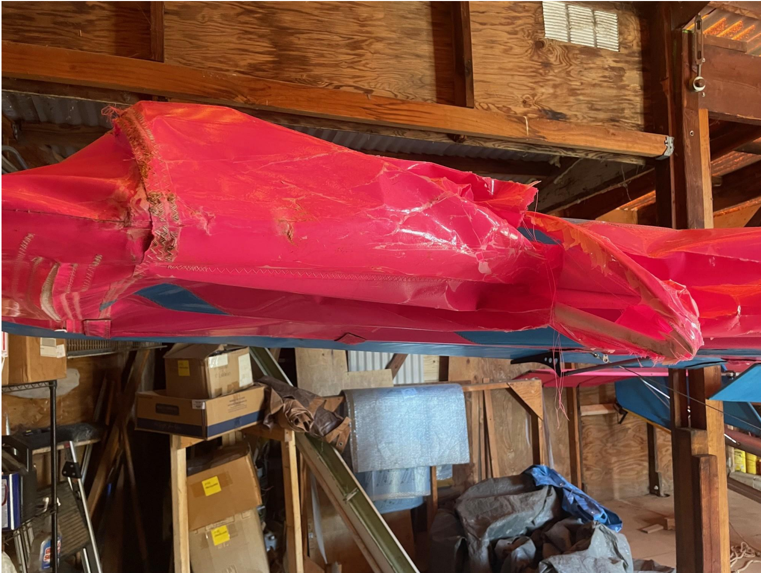
Photograph 2 - Damaged right wing (Courtesy of pilot)
