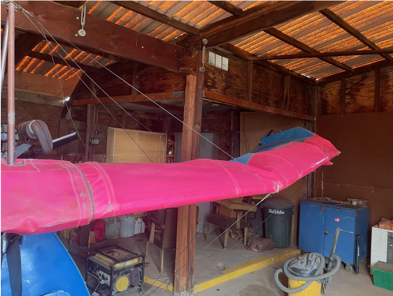
Photograph 3 - Damaged left wing (Courtesy of pilot)
