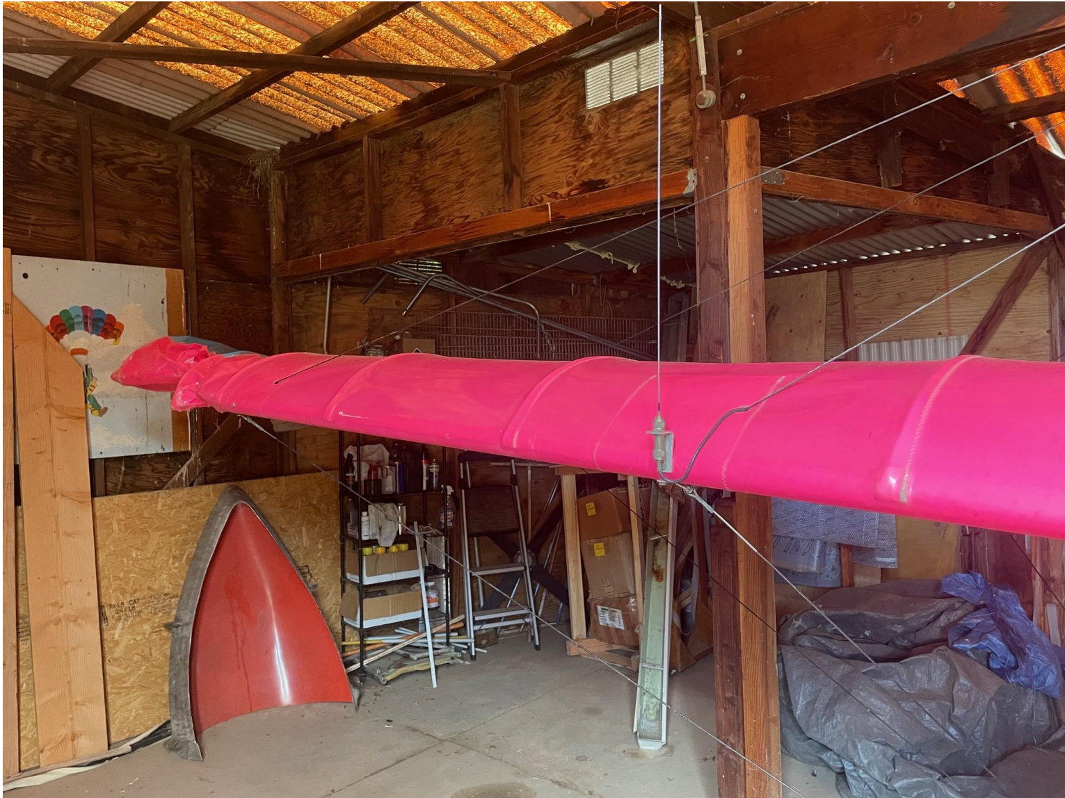
Photograph 1 - Damaged right wing (Courtesy of pilot)
