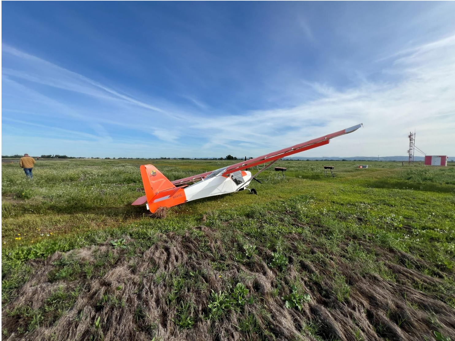
Photograph 2 - Right side view of airplane showing missing landing gear (Courtesy of airfield operations)
