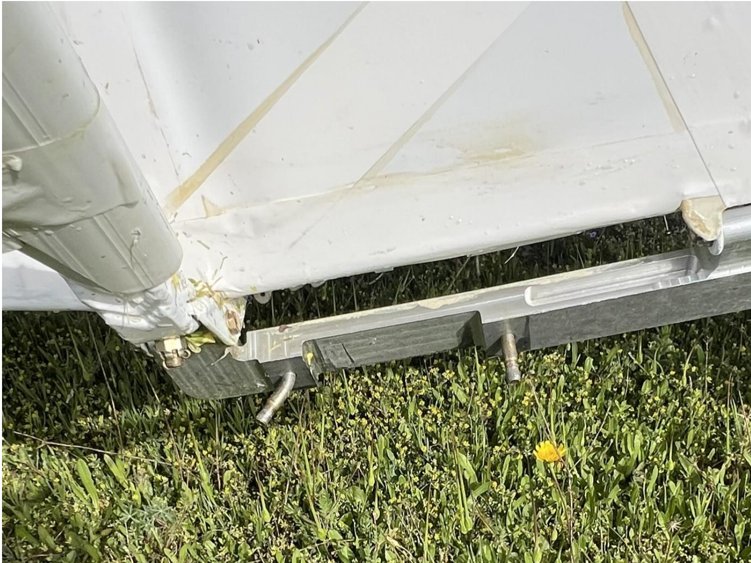
Photograph 4 - View of damage to landing gear attachment point (Courtesy of airfield operations)
