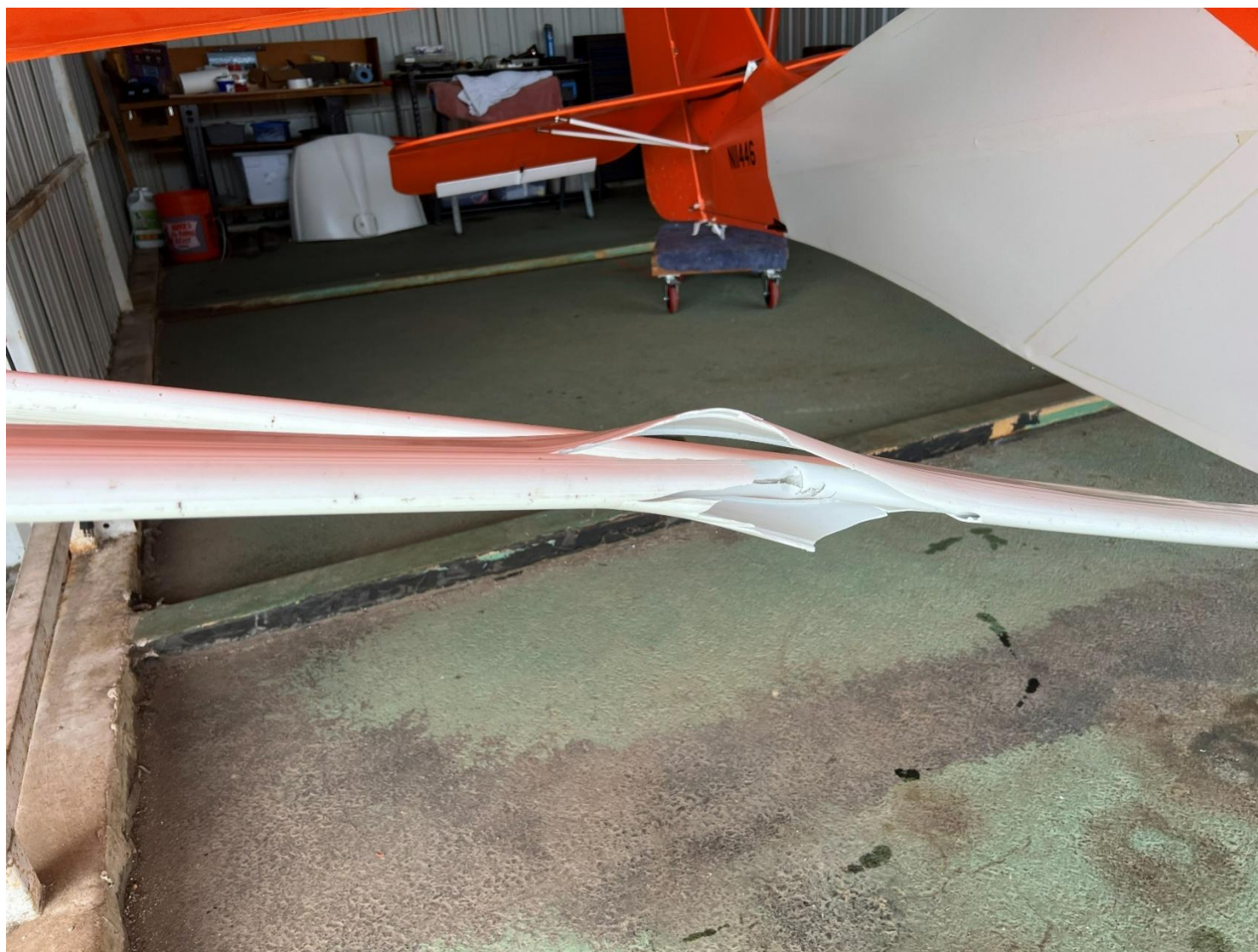
Photograph 3 - View of damage to right strut (Courtesy of airfield operations)
