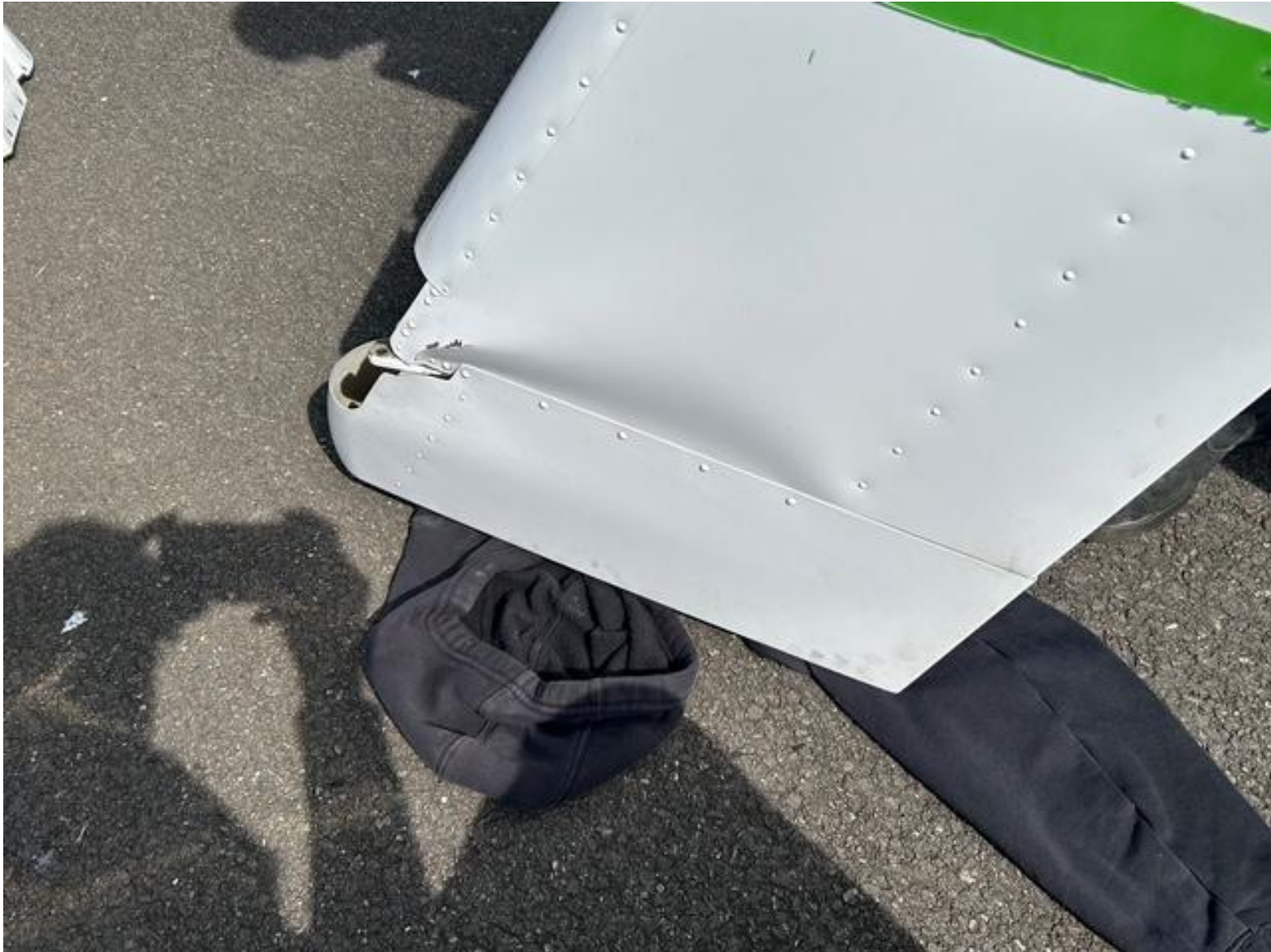
Photograph 1 - Damaged Rudder (Courtesy of flight school)
