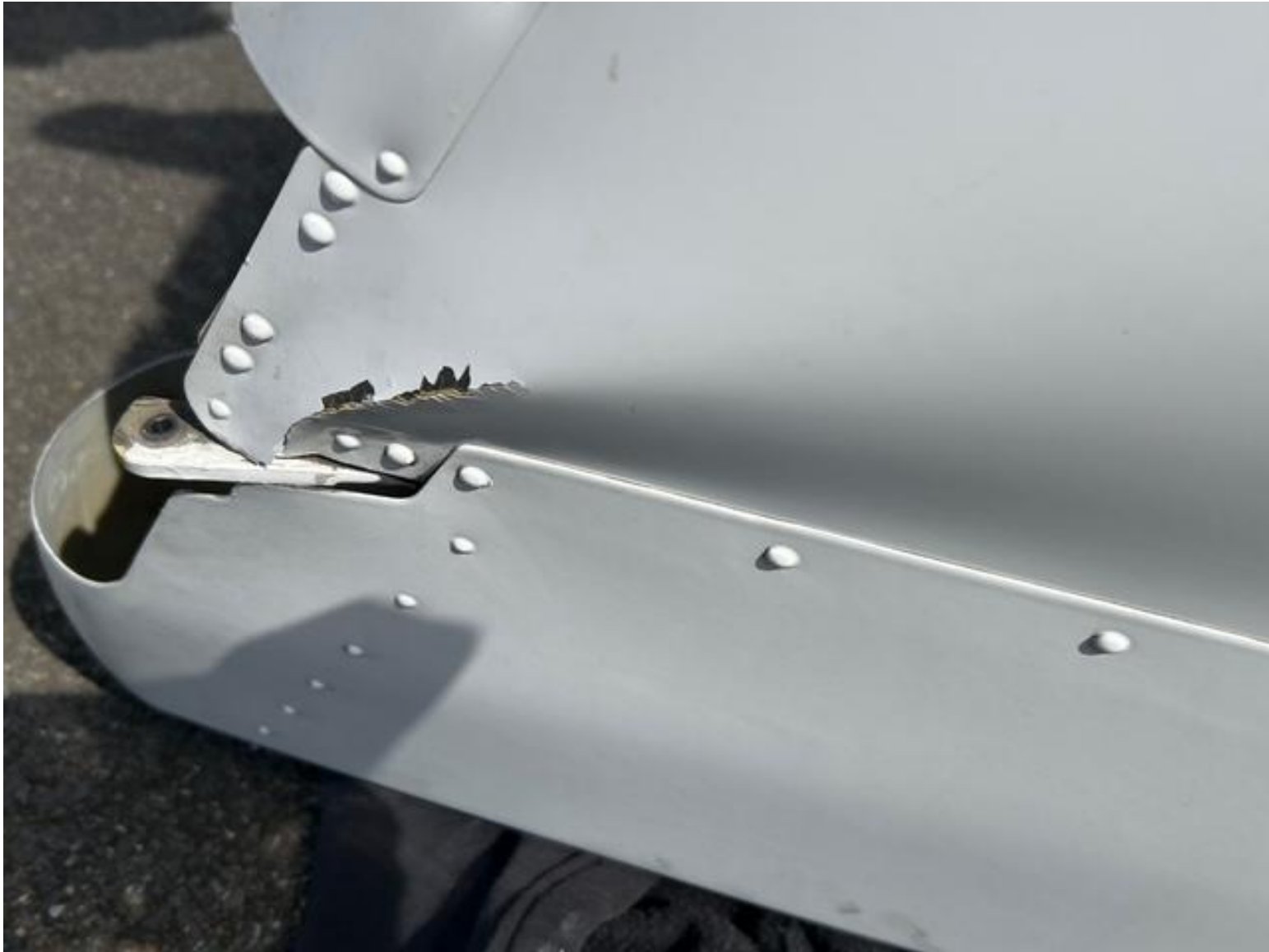
Photograph 2 - Damaged Rudder (Courtesy of flight school)
