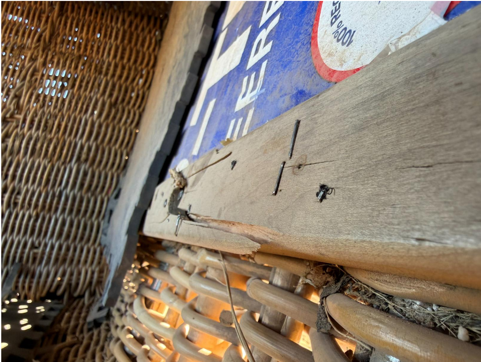
Photograph 5 - Fractured wood skid structure (Courtesy of pilot)
