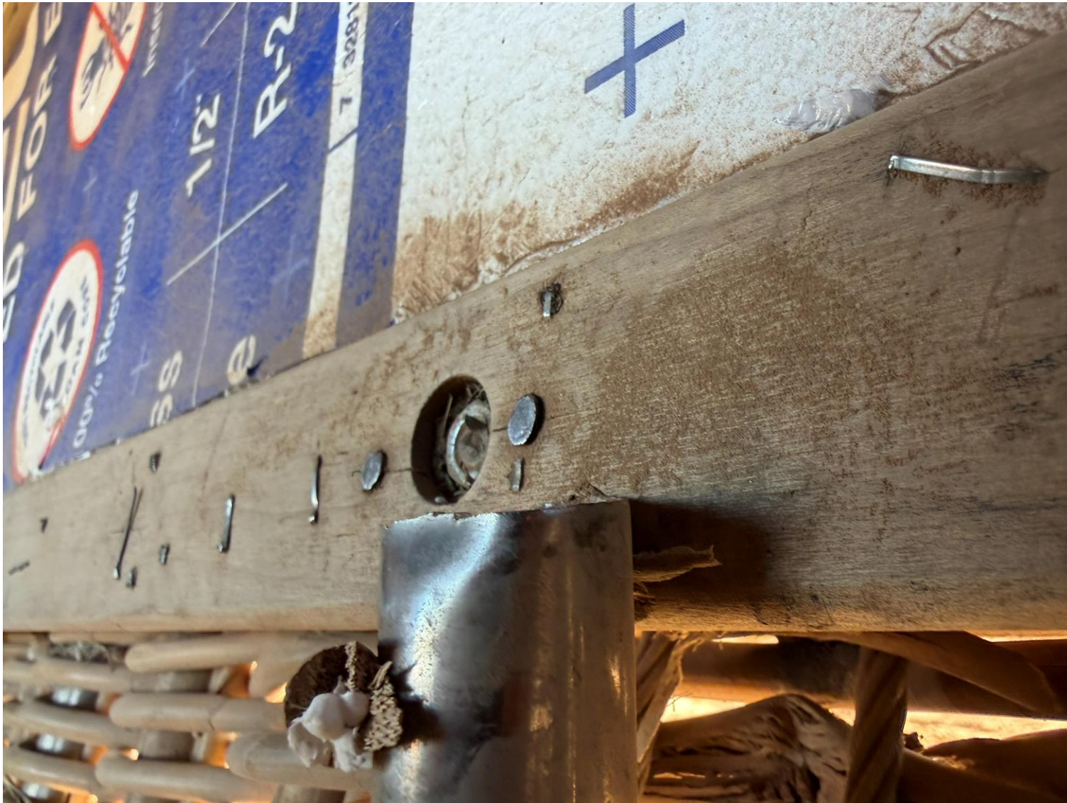
Photograph 2 - Fractured U-Tube (Courtesy of pilot)
