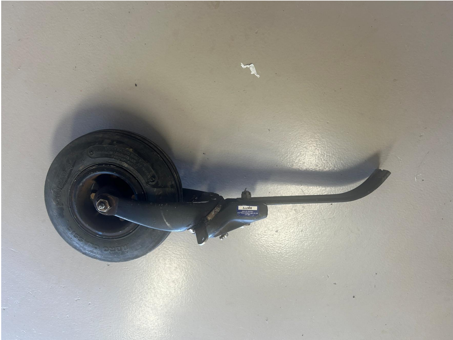
Photograph 5 - Pre-Accident Flight Separated Tailwheel Assembly (Courtesy of pilot)
