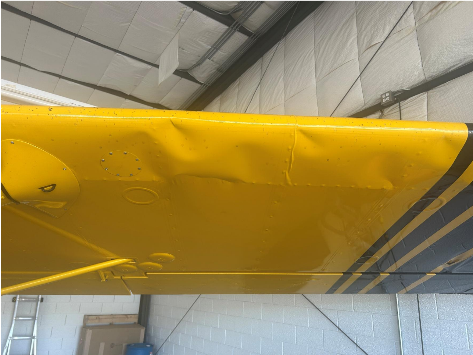
Photograph 2 - Accident Aircraft Damage - Wing (Courtesy of pilot)
