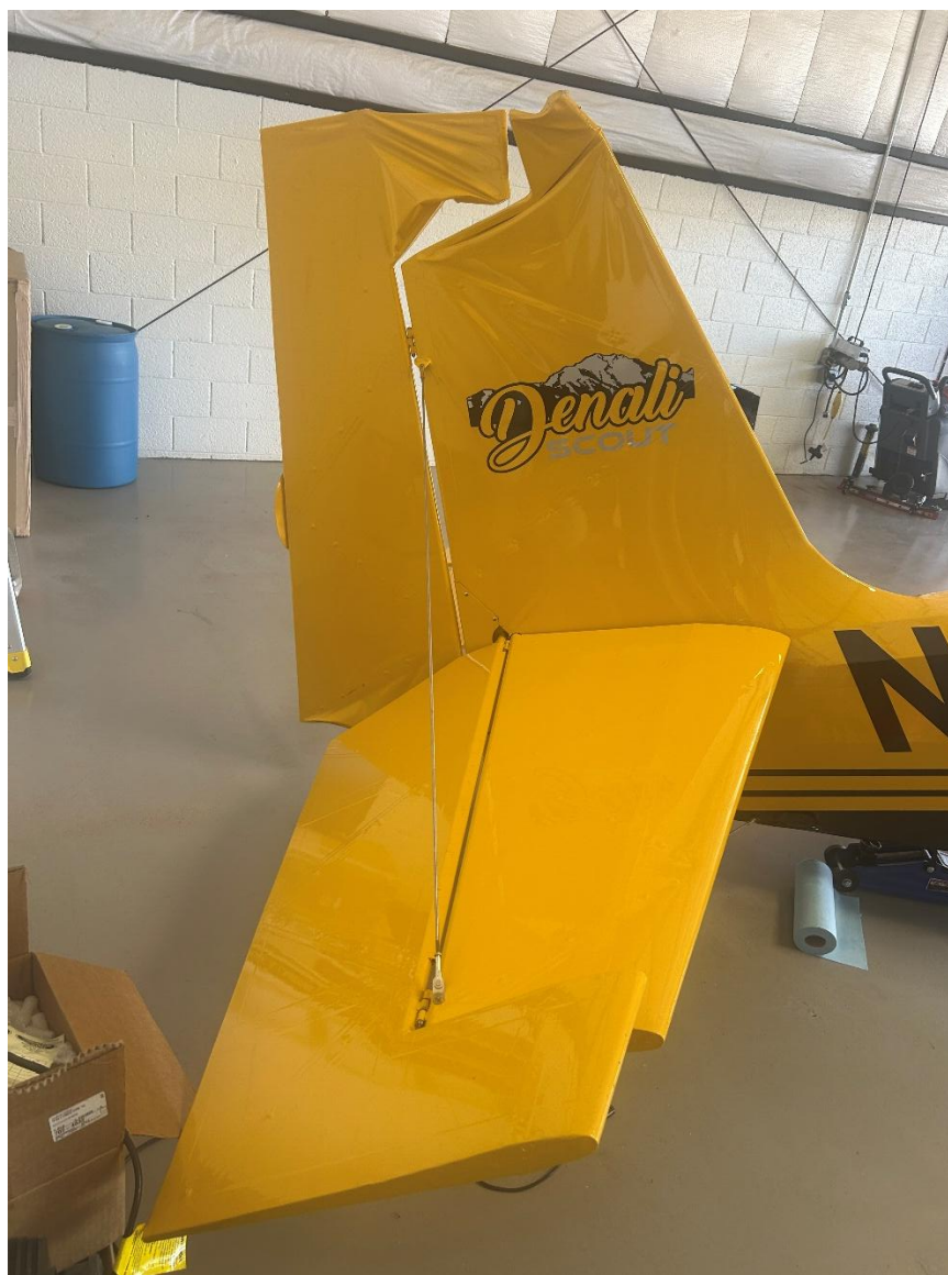
Photograph 3 - Accident Aircraft Damage - Empennage (Courtesy of pilot)
