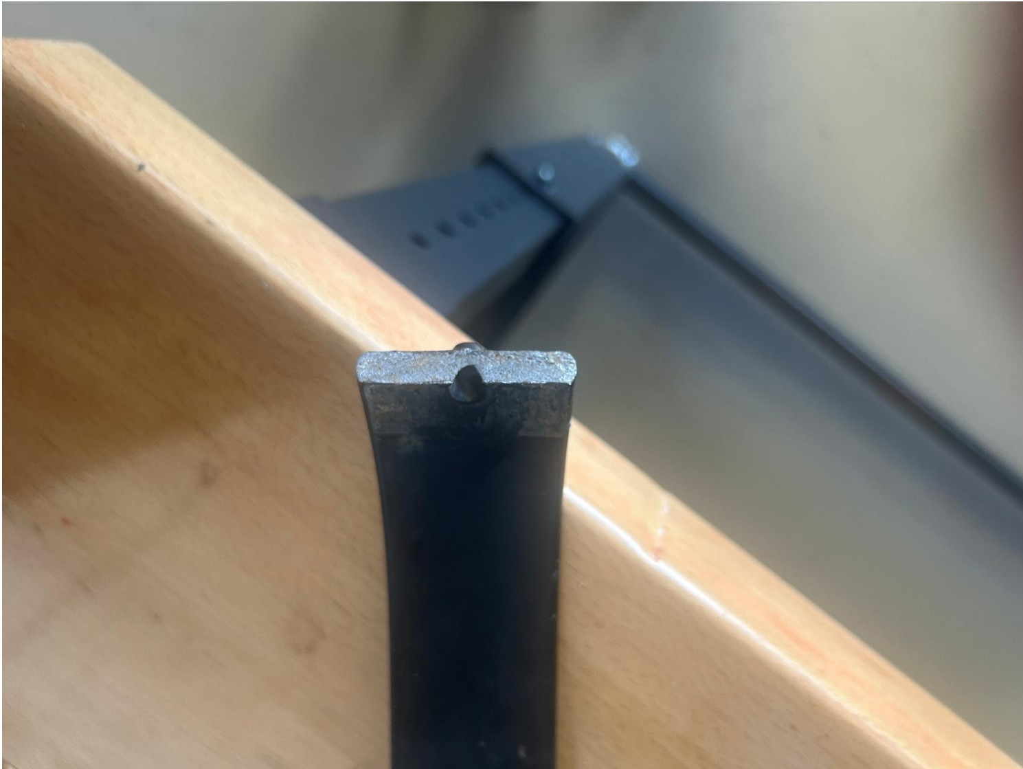
Photograph 5 - Pre-Accident Flight Separated Tailwheel Spring (Courtesy of pilot)
