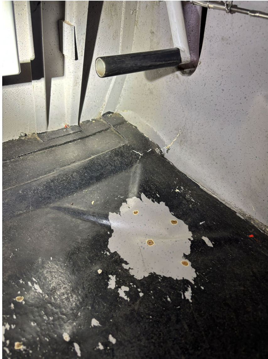
Photograph 4 - View of damage to the right-side floorboard (Courtesy of operator)
