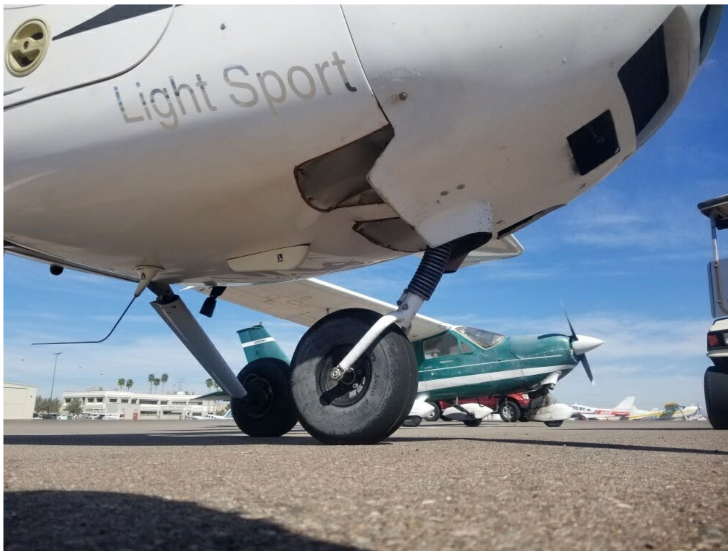
Photograph 2 - View of nose gear buckled (Courtesy of airport operations)
