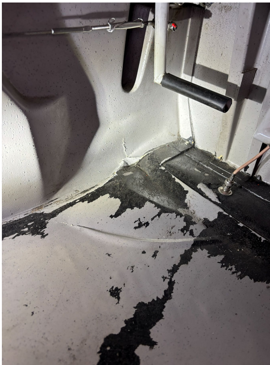
Photograph 5 - View of damage to left side floorboard (Courtesy of operator)
