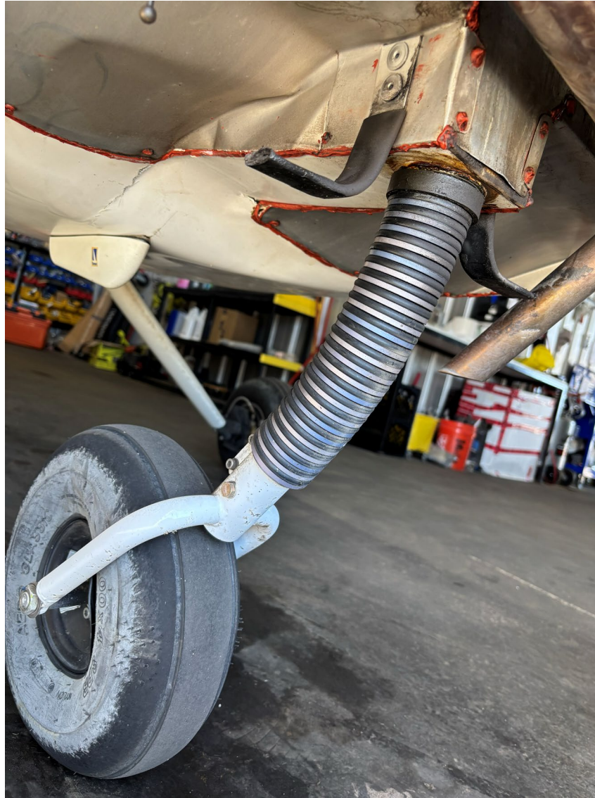
Photograph 3 - View of firewall and fuselage damage (Courtesy of operator)
