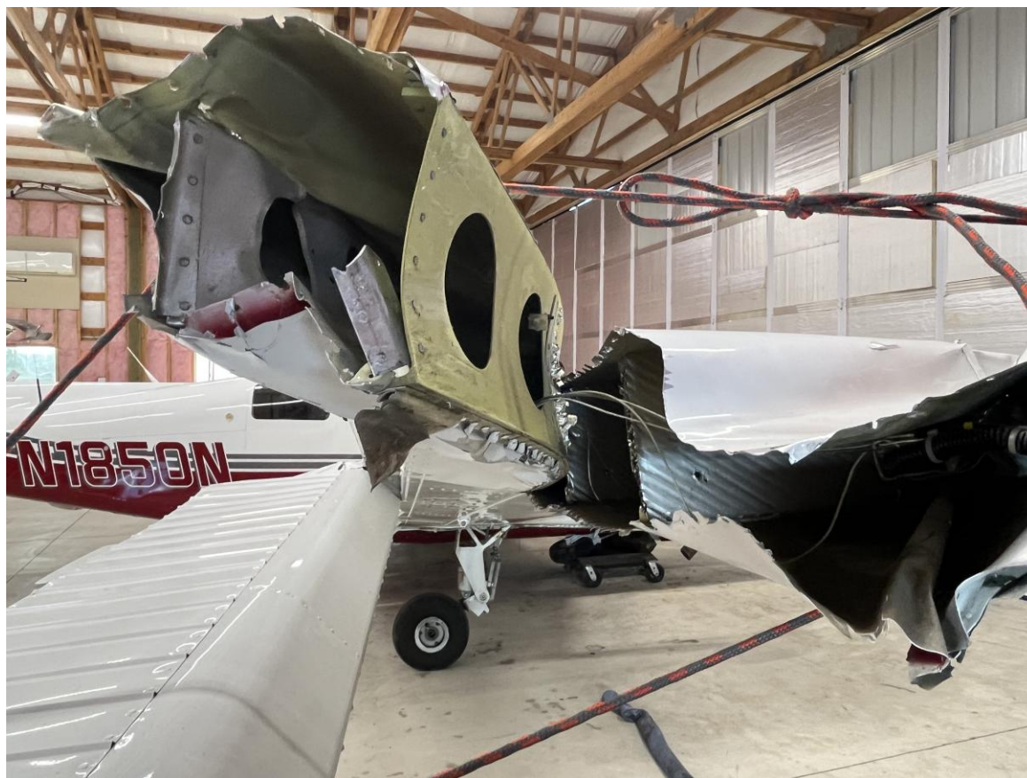
Photograph 2 - View of right wing damage (Courtesy of the Federal Aviation Administration)
