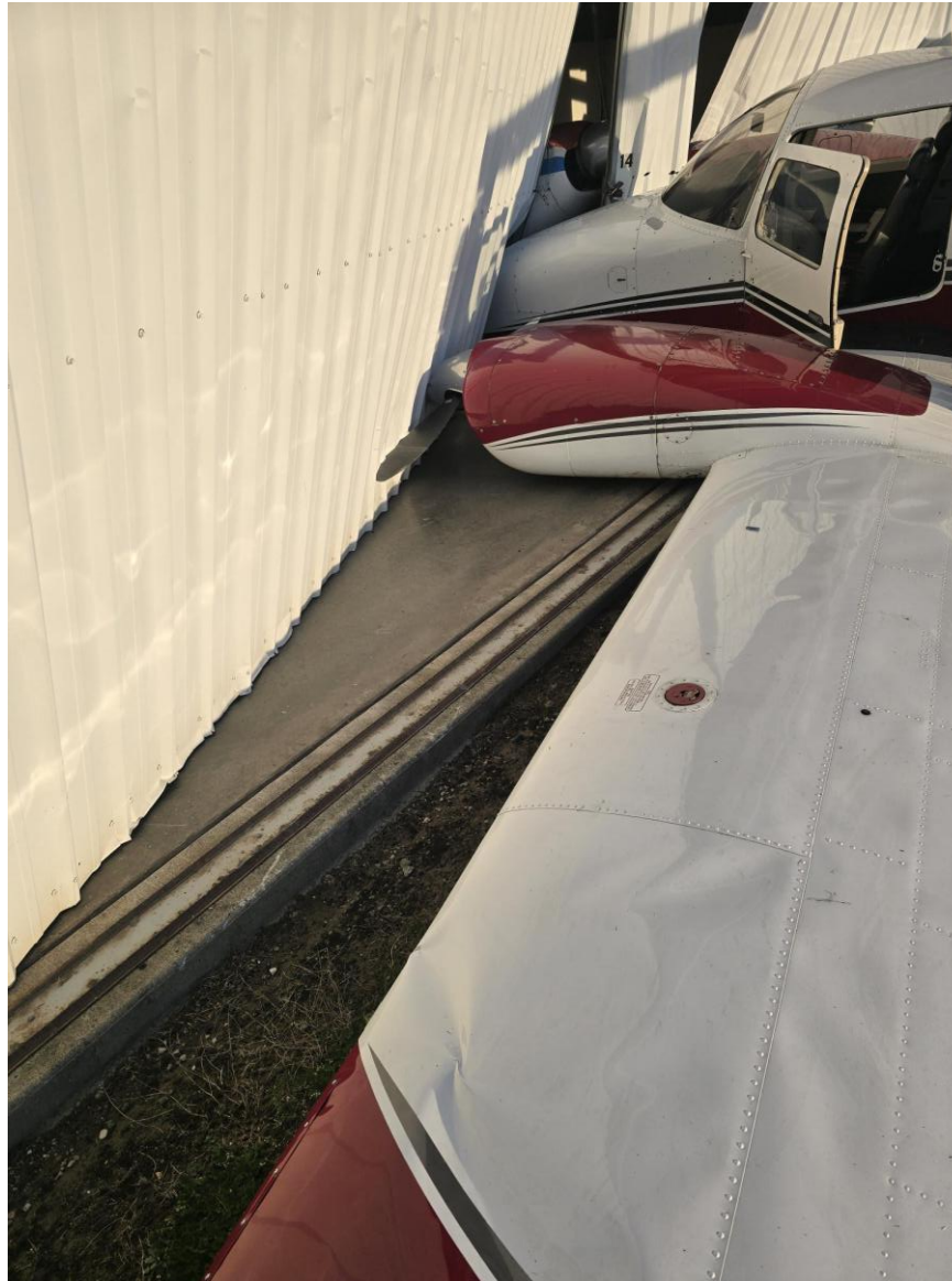
Photograph 4 - View of left wing damage (Courtesy of Airport Operations)
