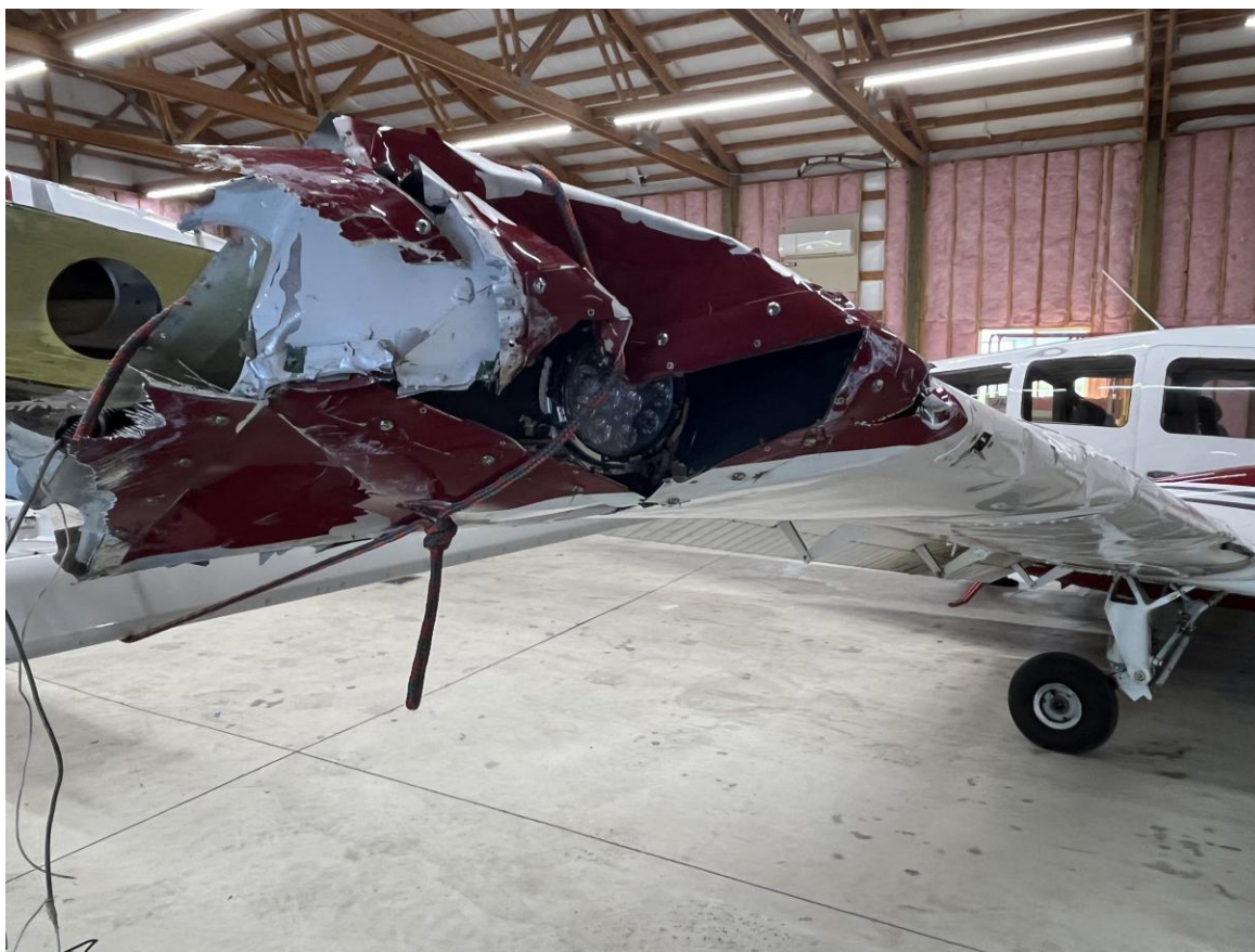
Photograph 1 - View of right wing damage (Courtesy of the Federal Aviation Administration)
