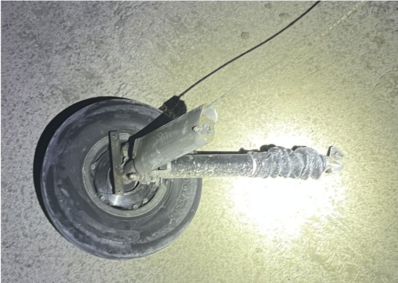
Photograph 2 - View of the left main landing gear attachment point separation (Courtesy of LEA)
