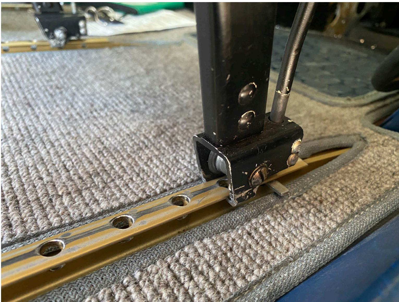
Photograph 4 - Right seat on rails, slid full forward (Courtesy of FAA)
