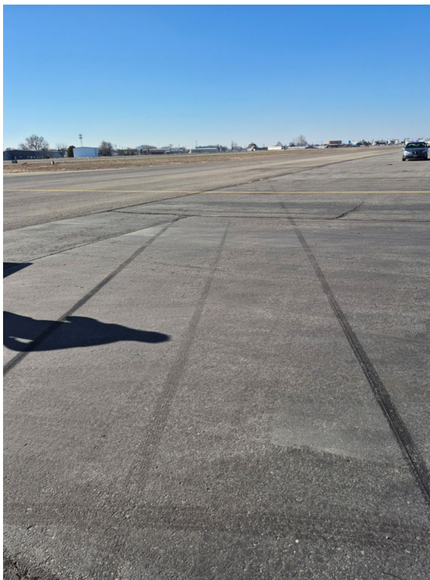
Photograph 3 - View showing tire skid marks on ramp (Courtesy of Pilot)
