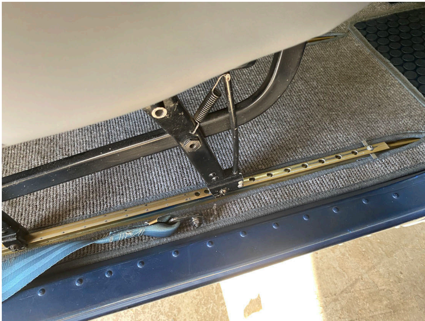
Photograph 5 - Right seat on seat rails (Courtesy of FAA)
