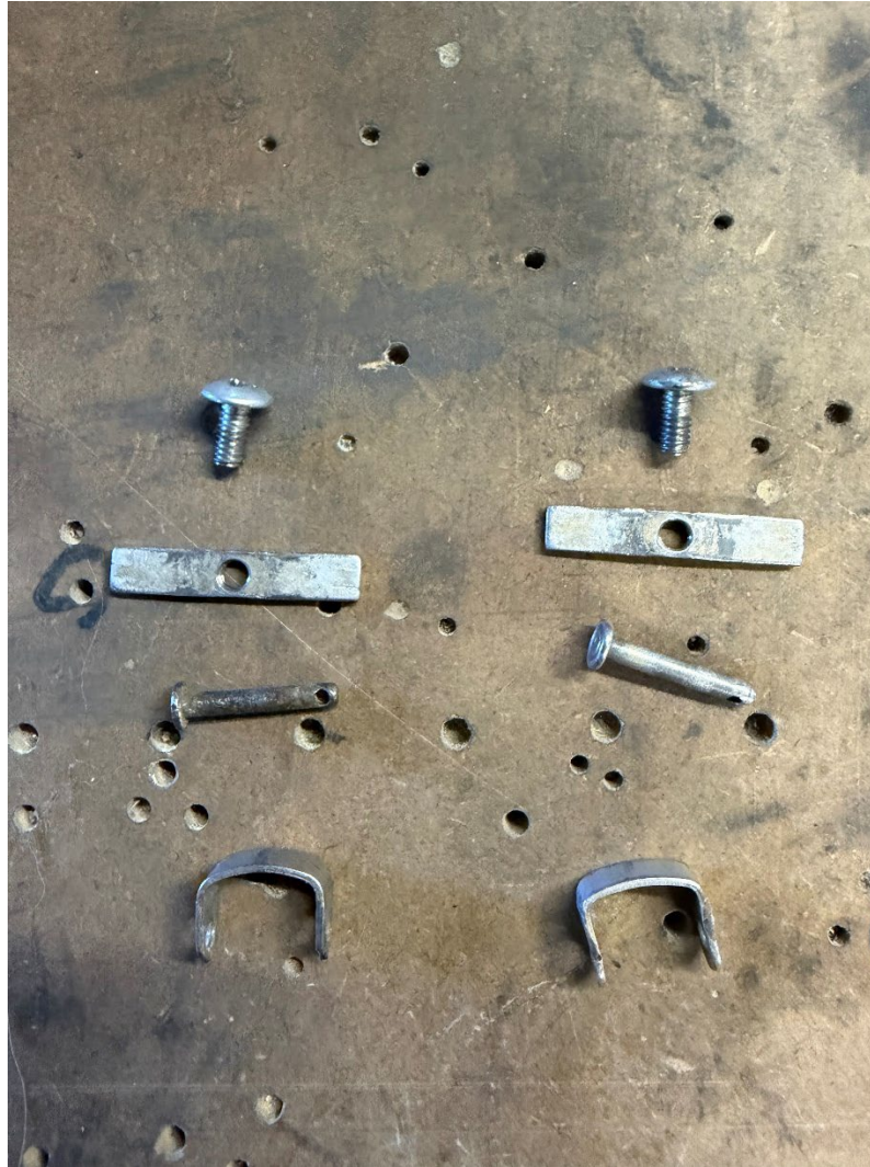
Photograph 6 - Right seat rail forward stop mounting hardware (Club maintenance director)
