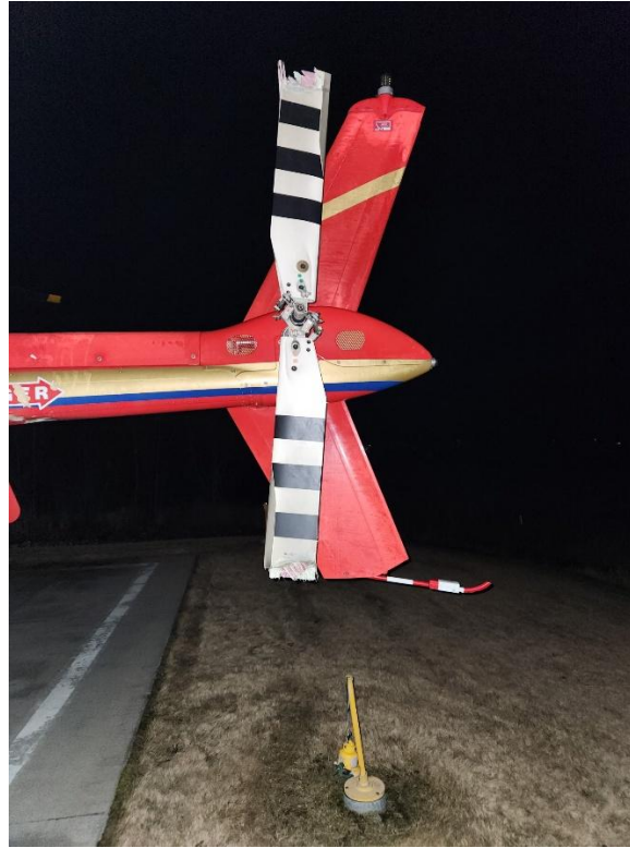
Photograph 4- View of tailboom, tail rotor, and light post damage (Courtesy of Pilot)
