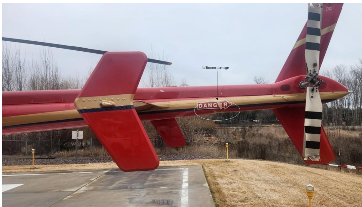
Photograph 1 - Side view of tailboom damage (Courtesy of Aircraft Operator)
