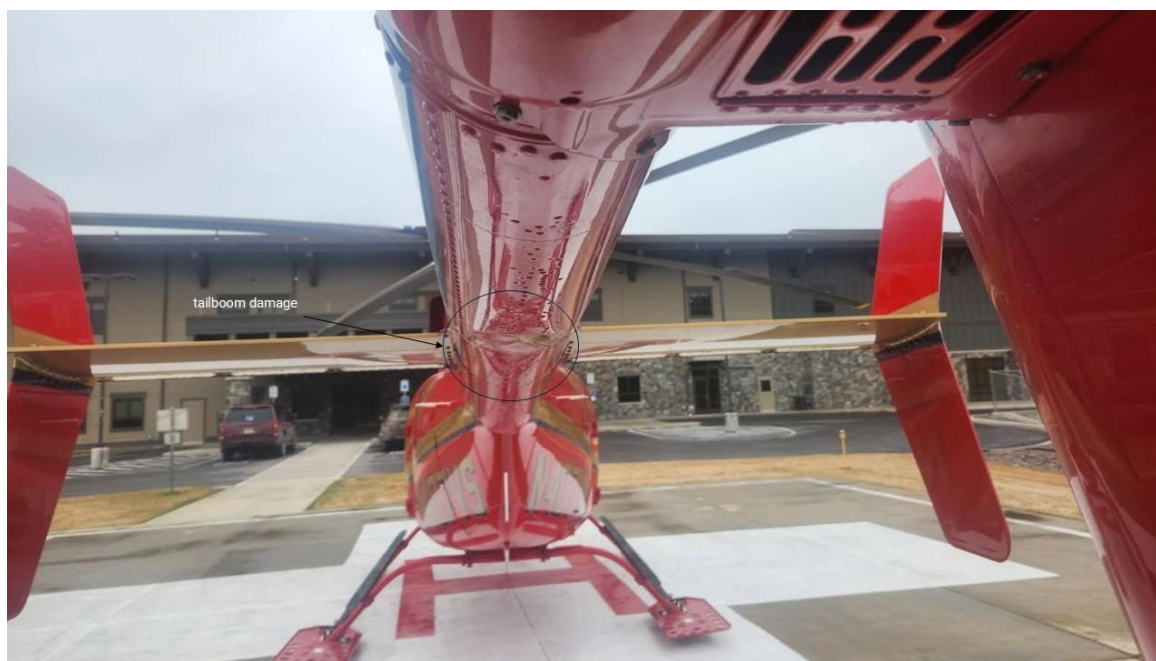
Photograph 3 - Rear view of tailboom damage (Courtesy of Aircraft Operator)
