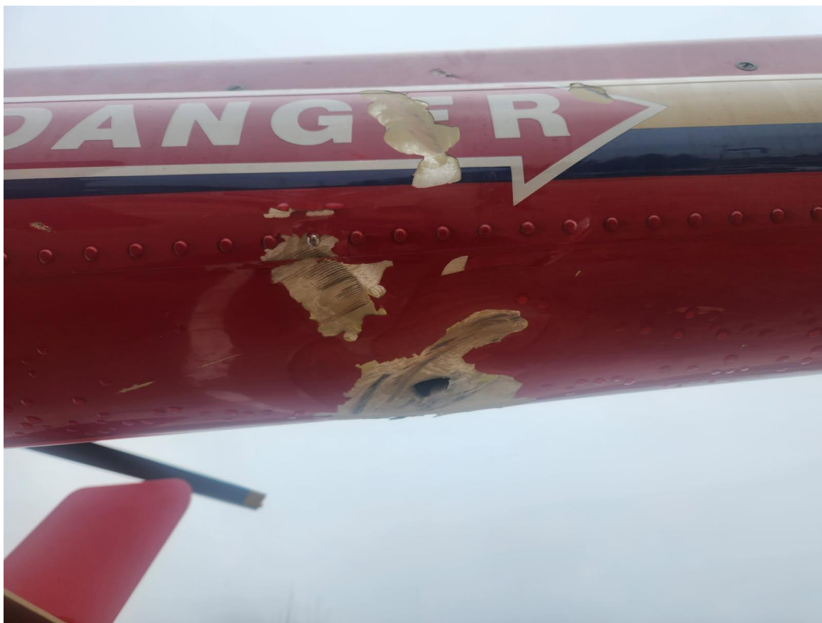
Photograph 2 - Bottom view of tailboom damage (Courtesy of Aircraft Operator)
