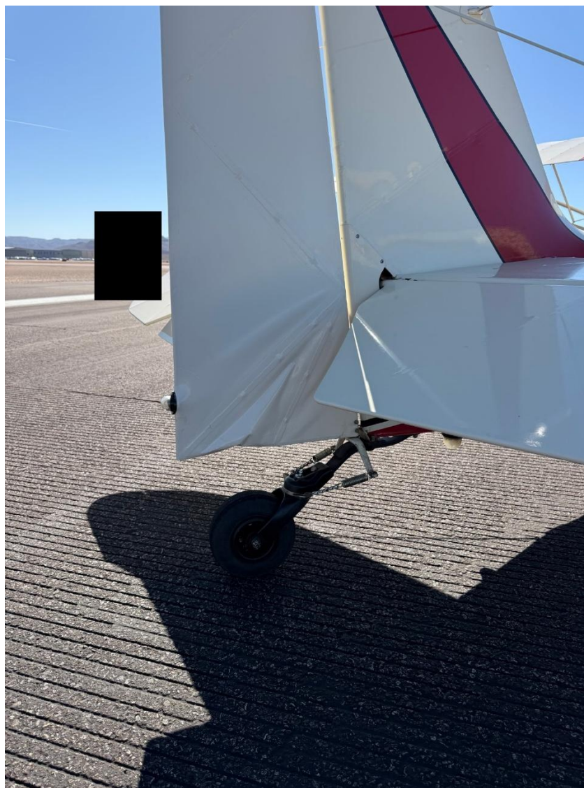
Photograph 1 - Damaged Rudder (Courtesy of KSGU Airport Operations)
