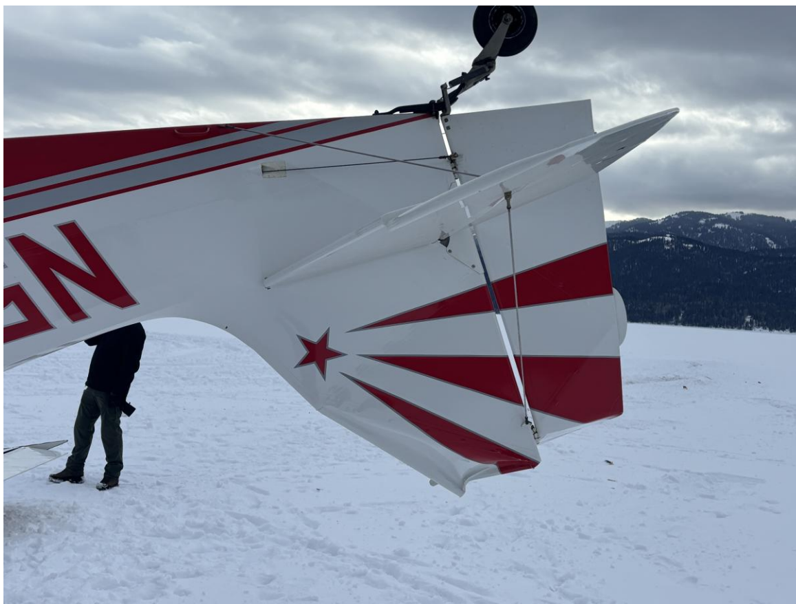
Photograph 3 - View of vertical stabilizer and rudder damage (Courtesy of Sheriff's Office)
