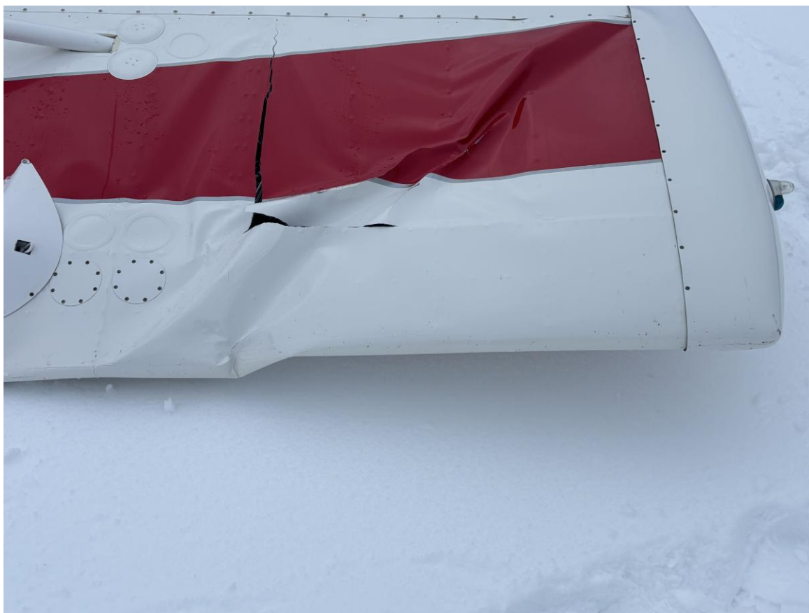
Photograph 4 - View of right wing damage (Sheriff's Office)
