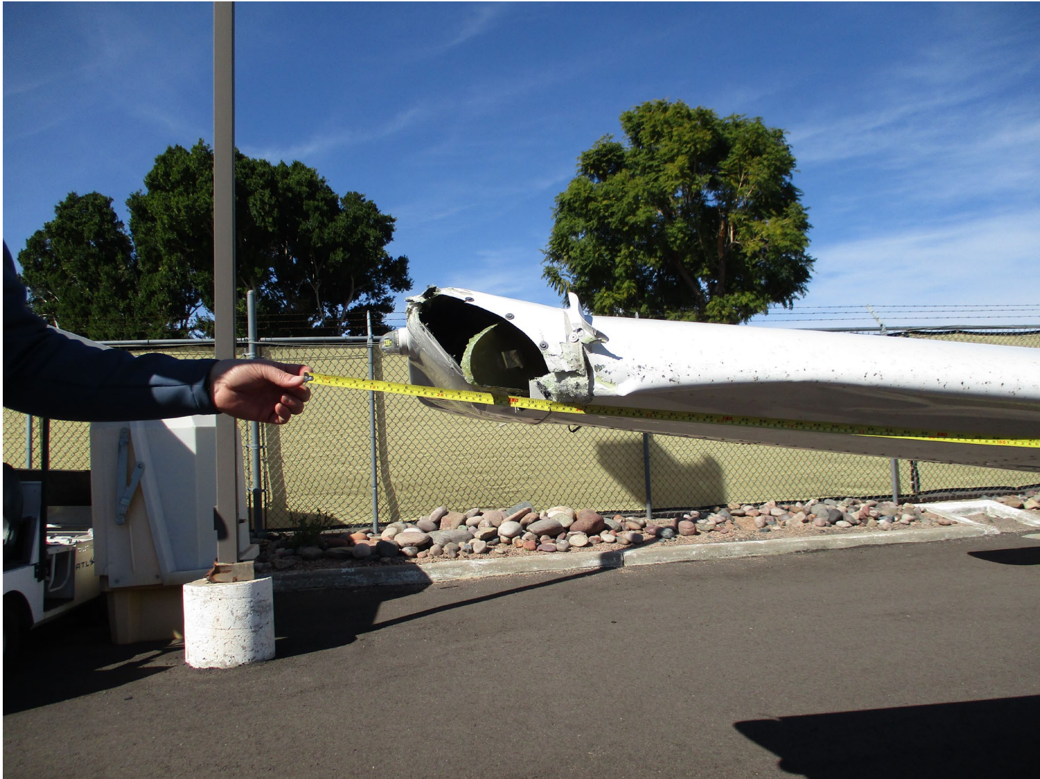
Photograph 5 - Right-wing leading-edge damage (courtesy of FAA)
