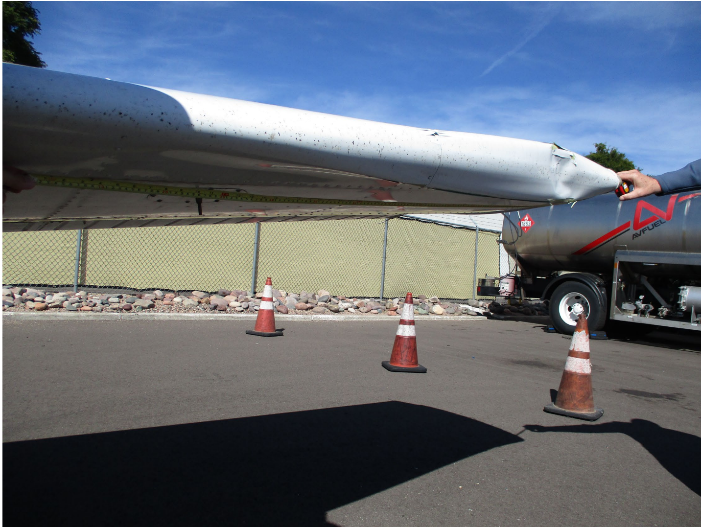
Photograph 3 - Left-wing leading-edge damage (courtesy of FAA)
