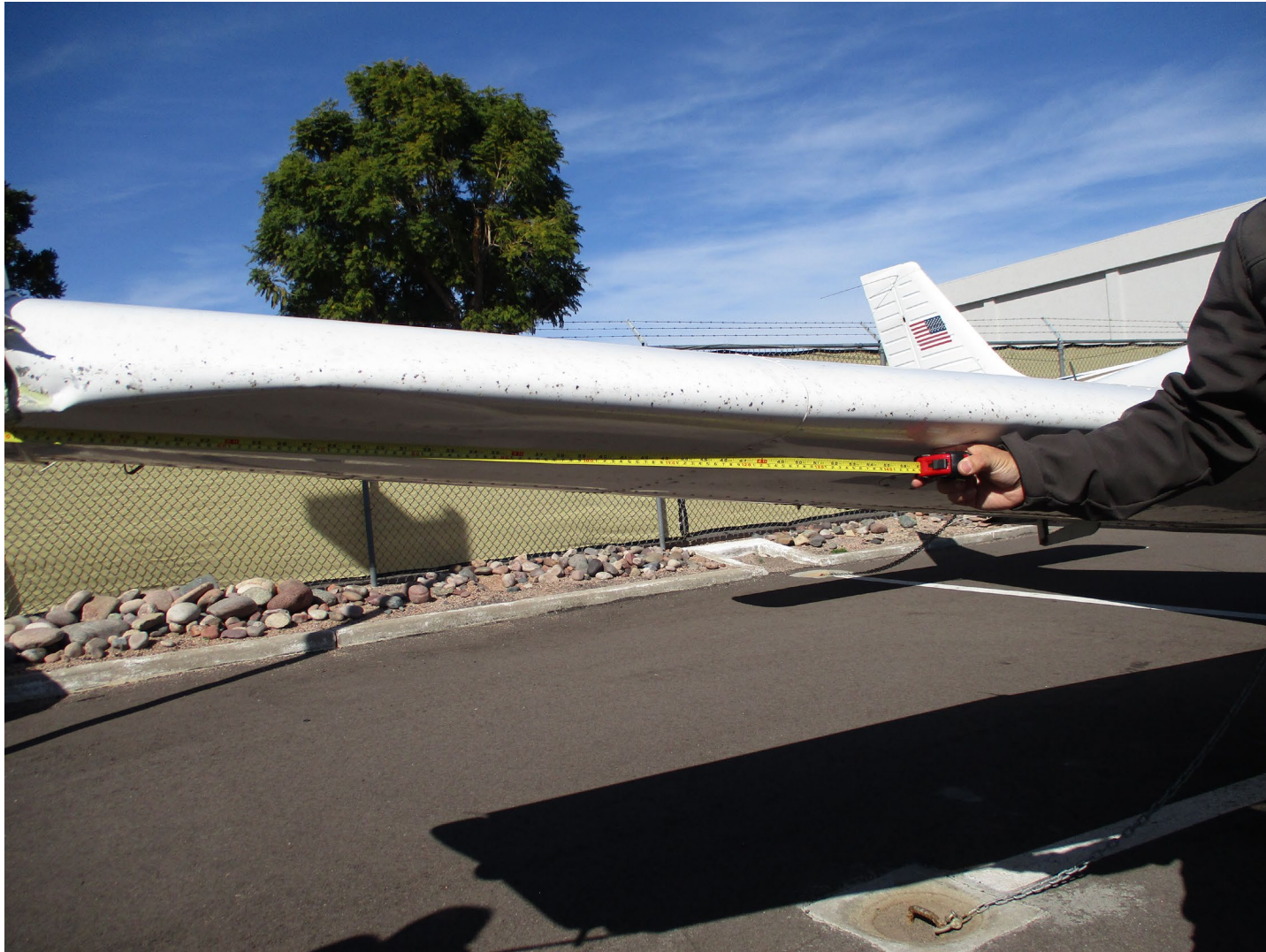
Photograph 4 - Right-wing leading-edge damage (courtesy of FAA)
