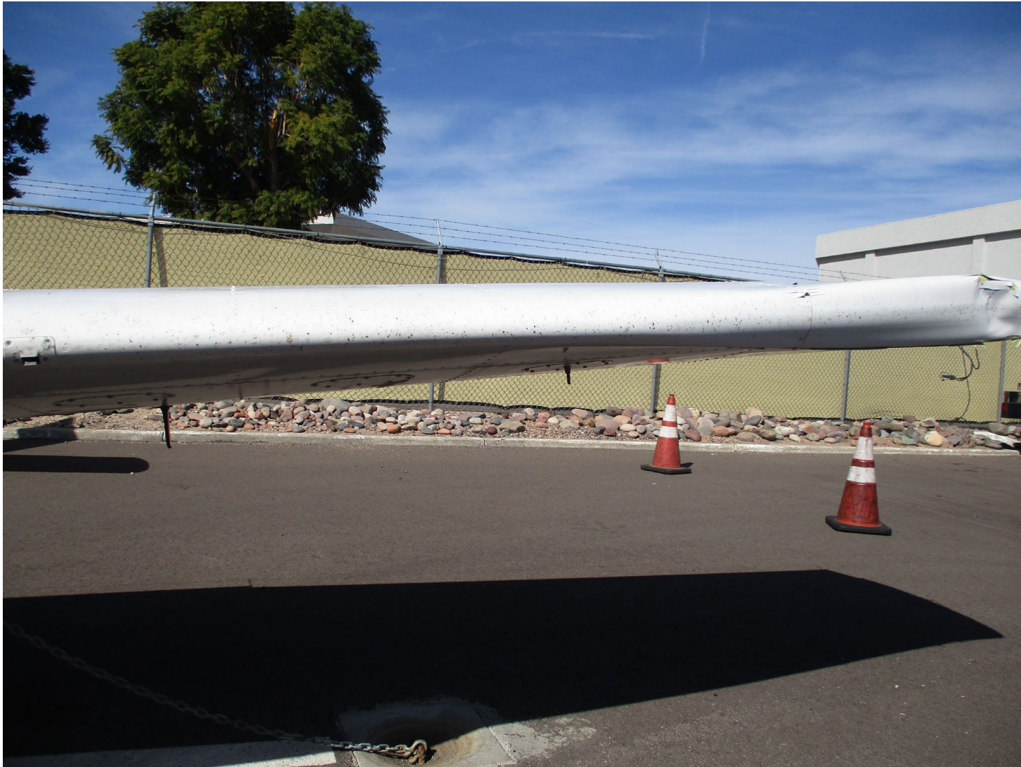
Photograph 2 - Left-wing leading-edge damage (courtesy of FAA)
