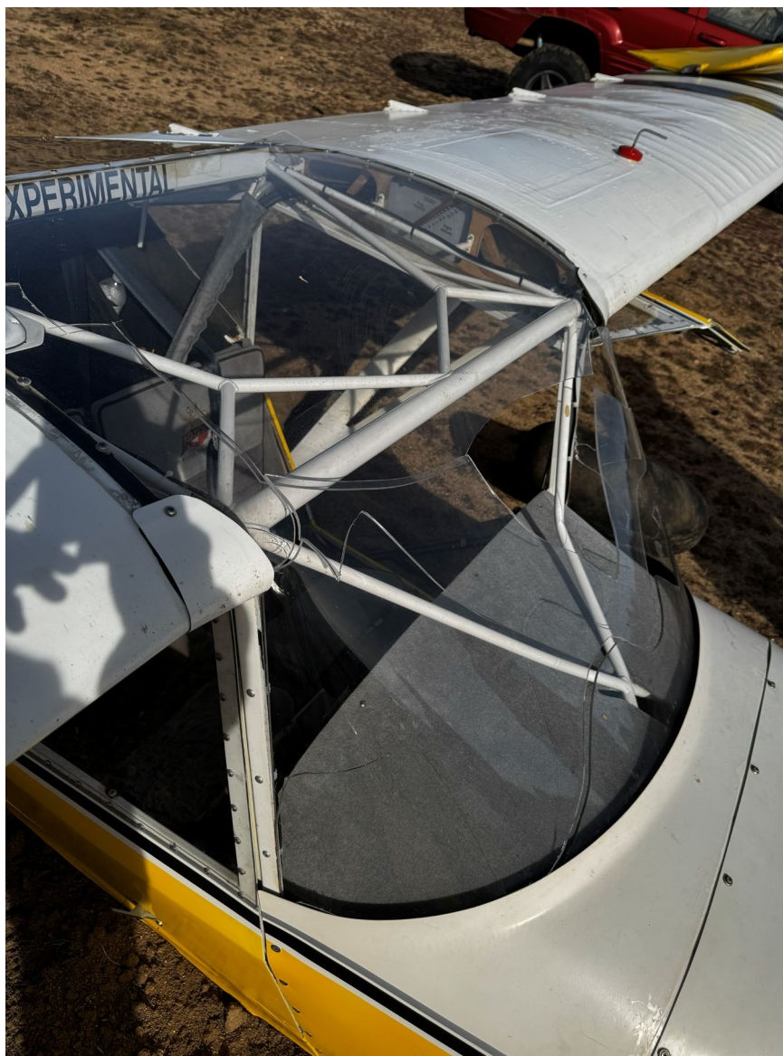
Photograph 4 - View of bent fuselage tube (Courtesy of Pilot)
