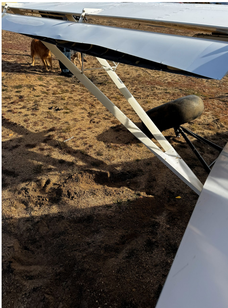
Photograph 3 - View of left flaperon damage (Courtesy of Pilot)
