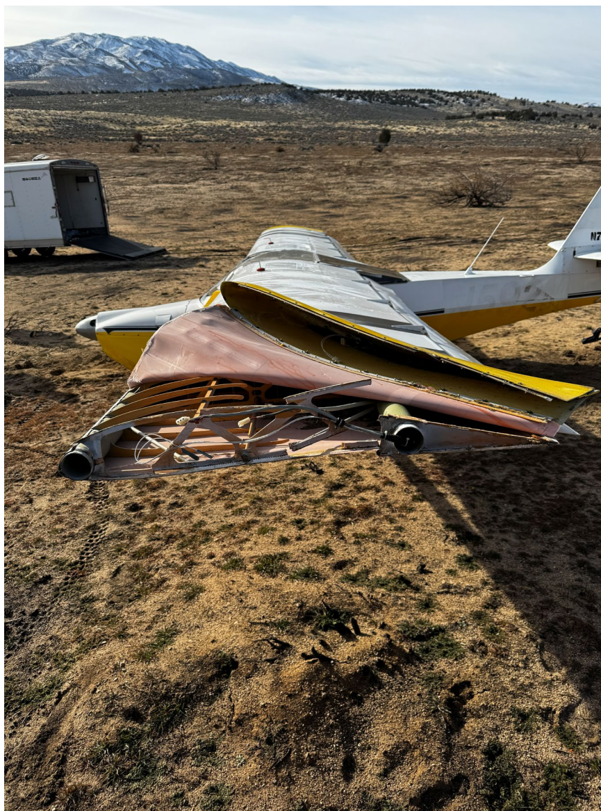
Photograph 2 - View of left-wing damage (Courtesy of Pilot)
