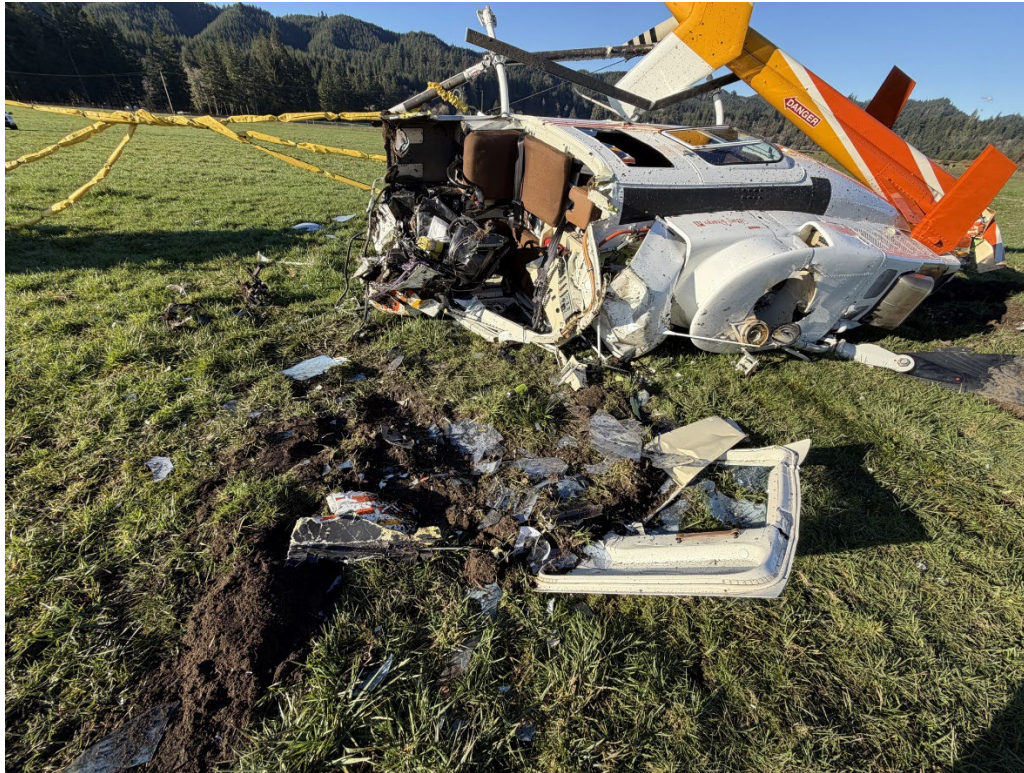
Photograph 2 - Helicopter wreckage as viewed from the top front side with nylon cord wrapped around right skid. (Courtesy of Operator).
