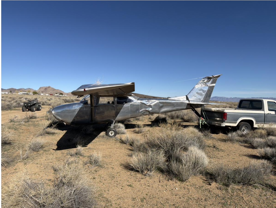
Photograph 1 - View of aft fuselage damage (Courtesy of local law enforcement)
