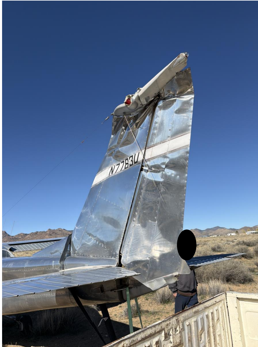
Photograph 2 - View of vertical stabilizer / rudder damage (Courtesy of local law enforcement)
