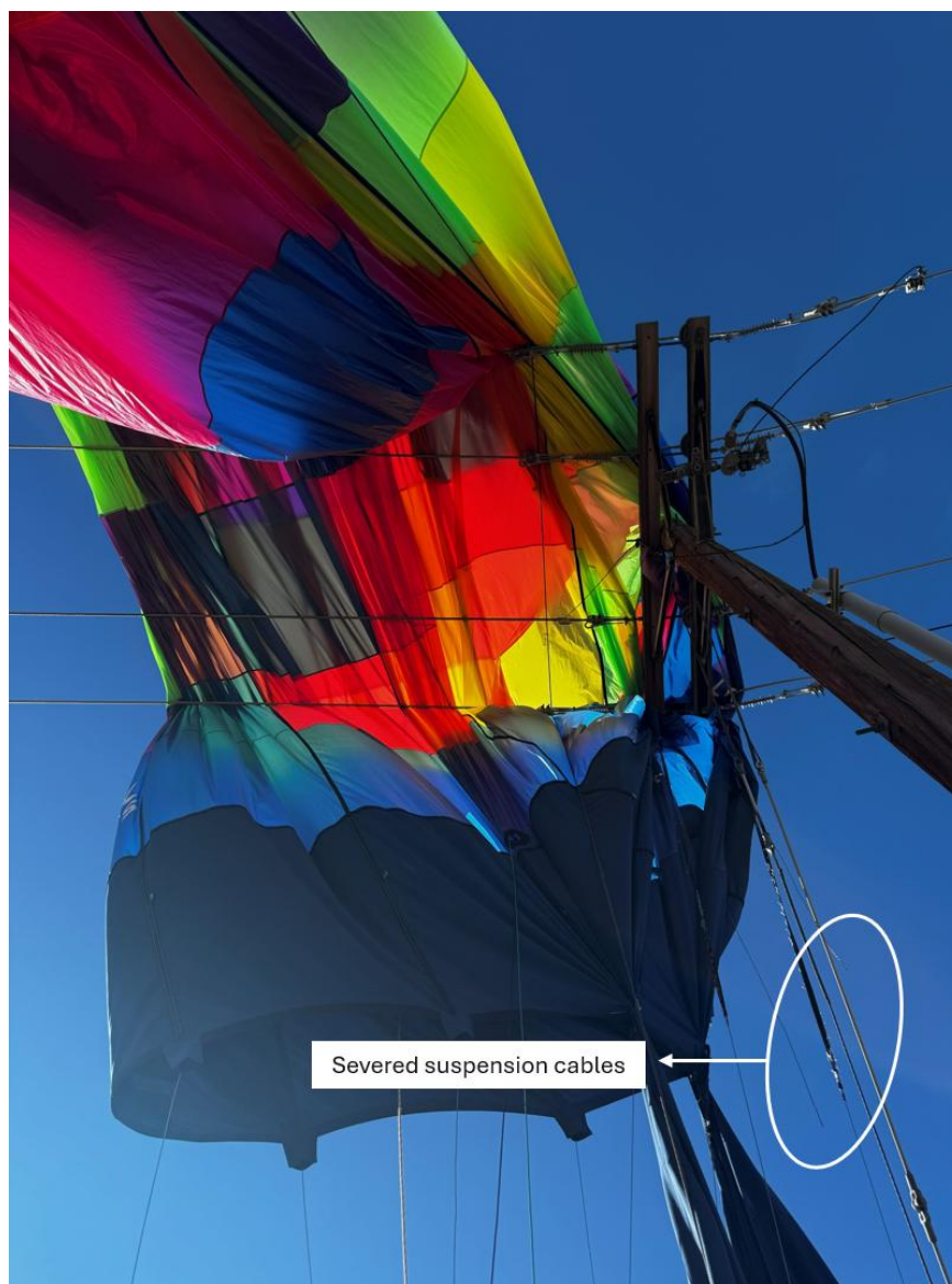
Photograph 2 - View of severed suspension cables. (Courtesy of LEO)
