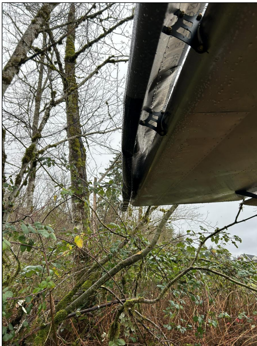
Photograph 5 - Accident site, right wing damage. (Courtesy of the Owner)
