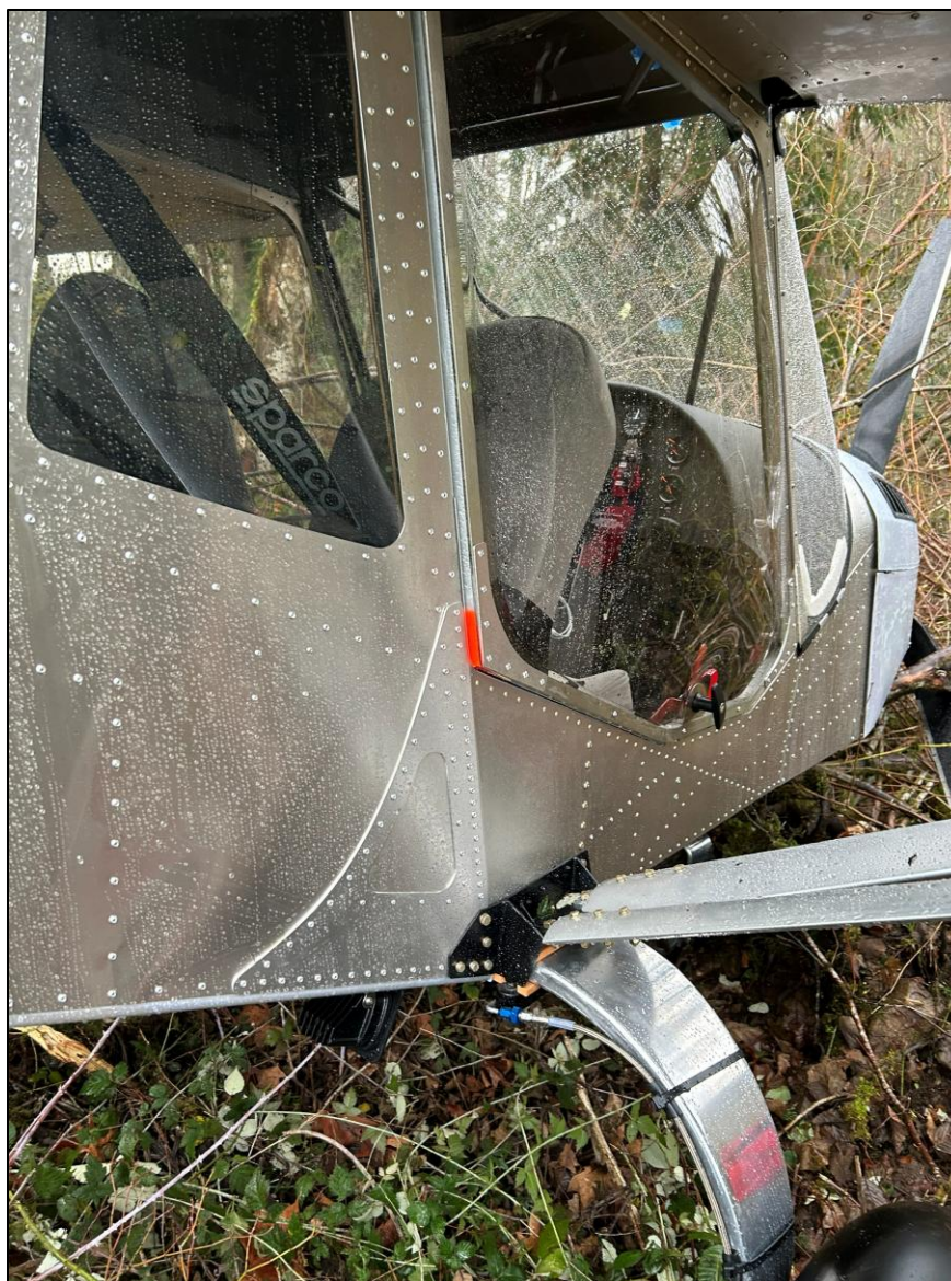
Photograph 4 - Accident site, fuselage damage. (Courtesy of the Owner)
