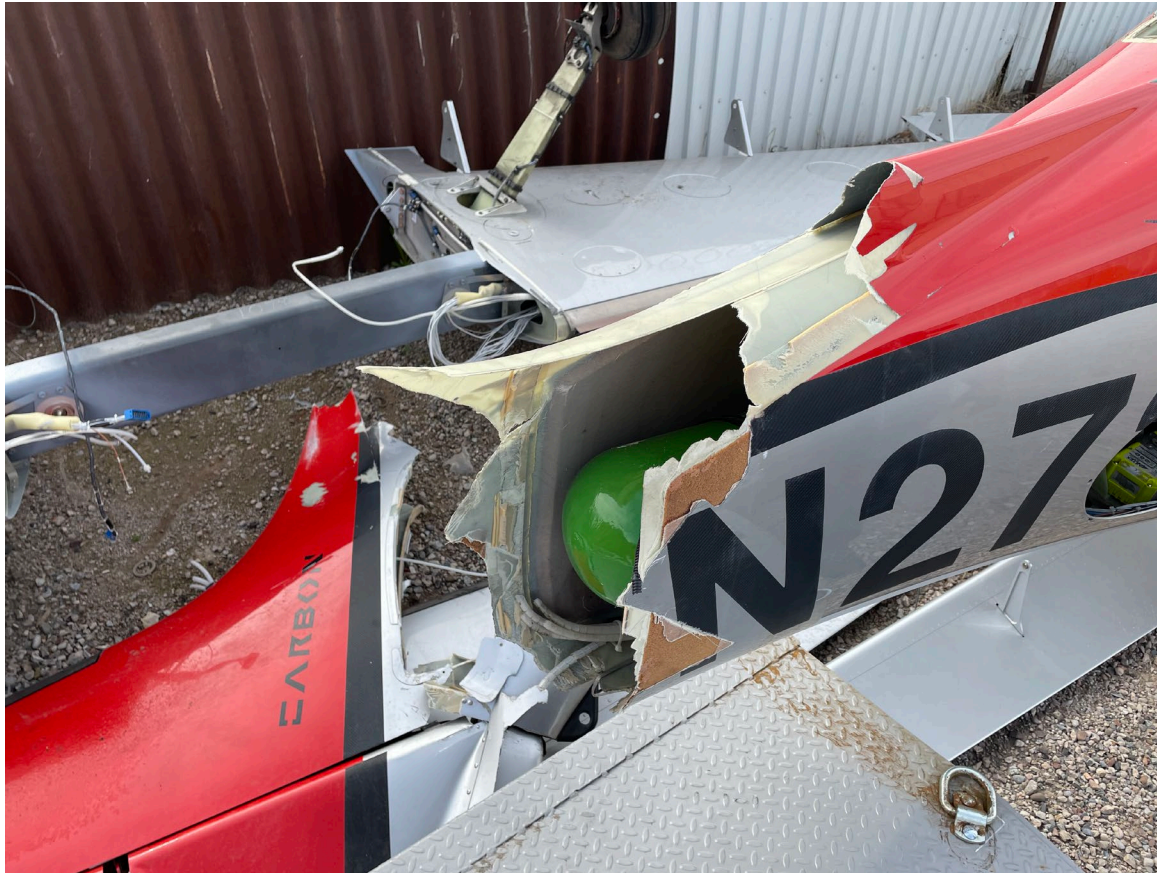
Photograph 3 - View of fractured fuselage (Courtesy of NTSB)
