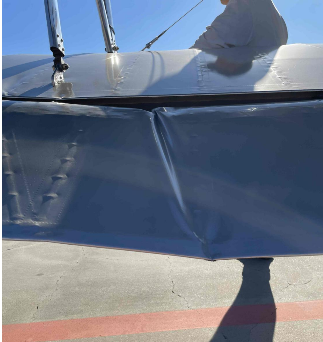
Photograph 2 - Lower left aileron damage (Courtesy of KSEE Airport Ops)
