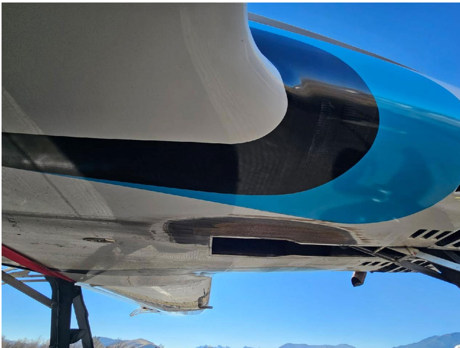
Photograph 2 - Carbon Fiber Abrasion right of nose-gear (courtesy of airport operations director)
