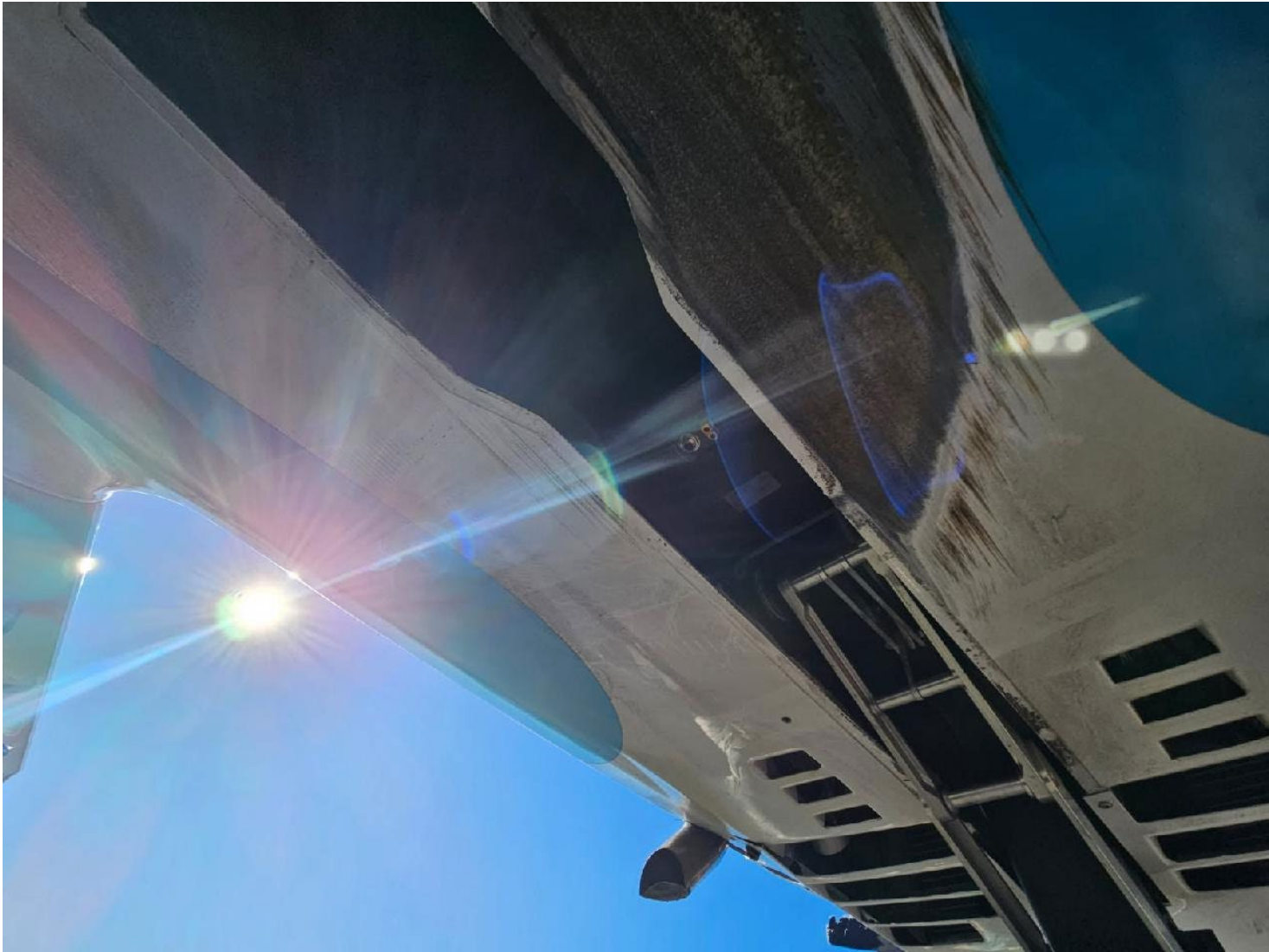
Photograph 1 - Carbon Fiber Abrasion right of nose-gear (courtesy of airport operations director)
