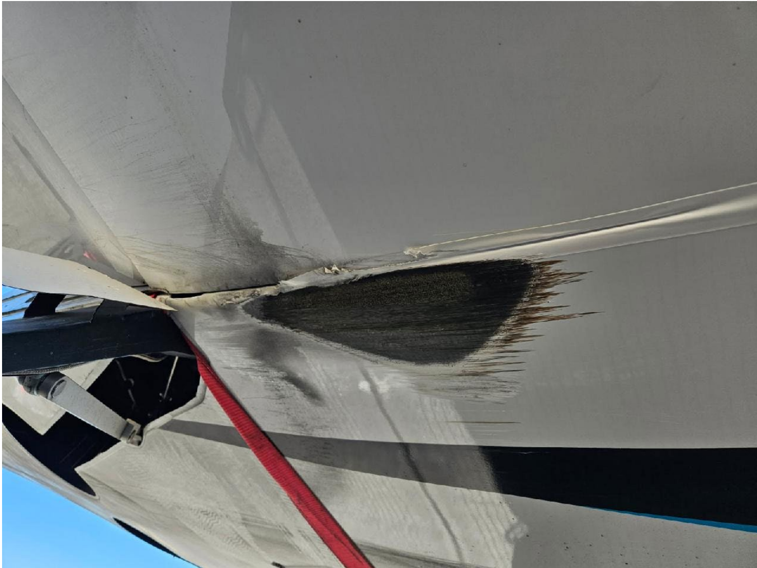
Photograph 4 - Carbon Fiber Abrasion on belly (courtesy of airport operations director)
