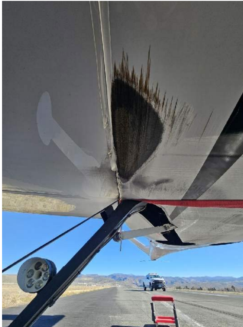
Photograph 6 - Carbon Fiber Abrasion on belly (courtesy of airport operations director)
