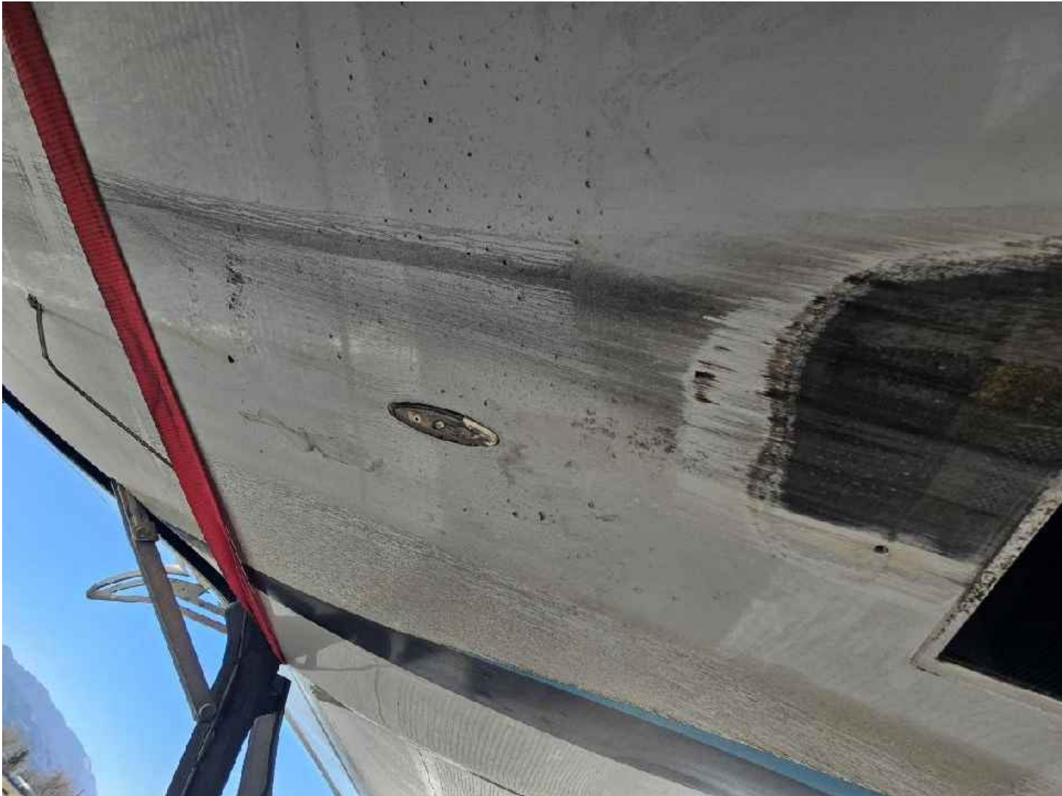
Photograph 3 - Carbon Fiber Abrasion on belly (courtesy of airport operations director)
