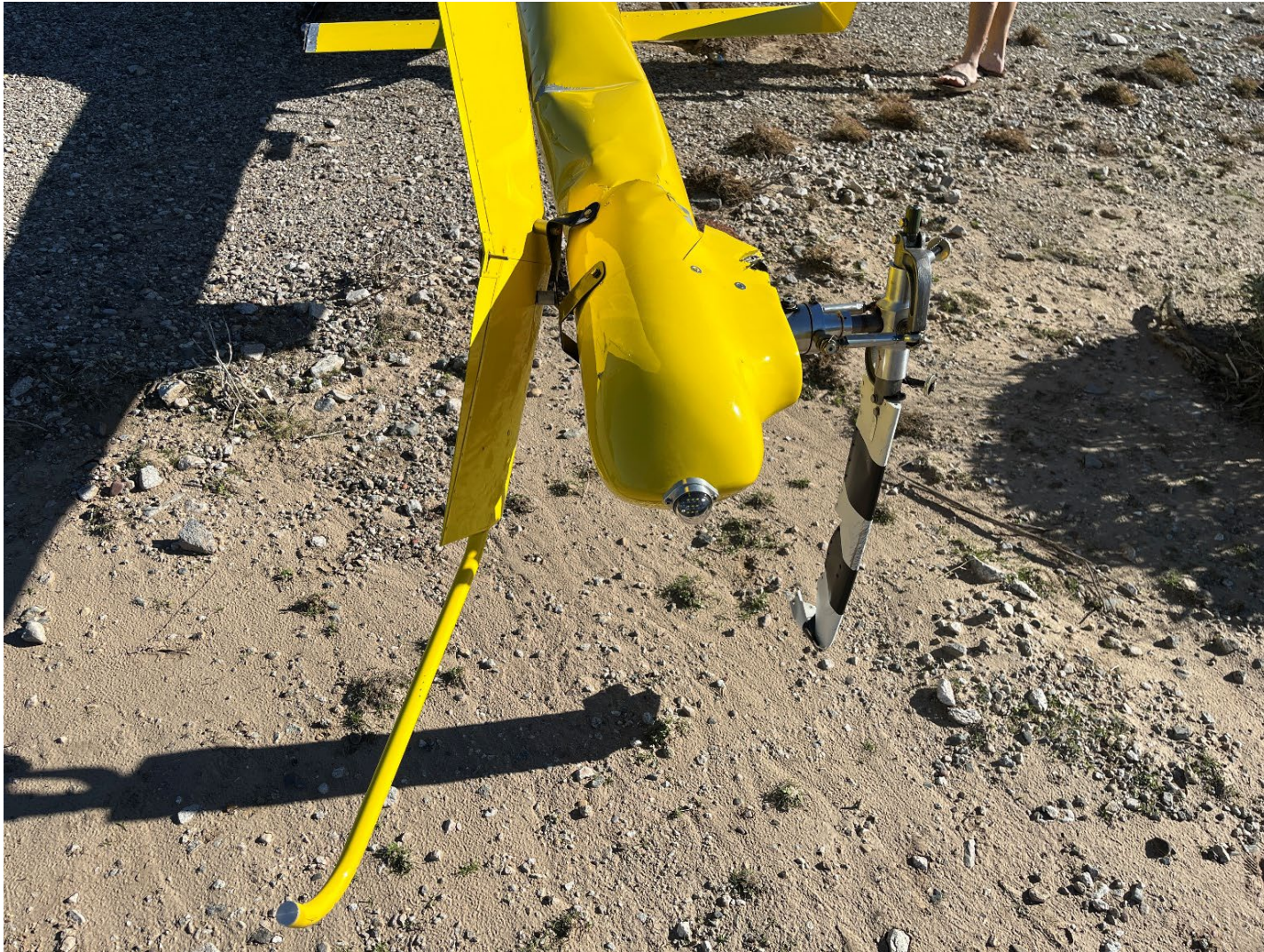
Photograph 2 - Damage to tail rotor blades (Courtesy of San Bernardino County Sheriff)
