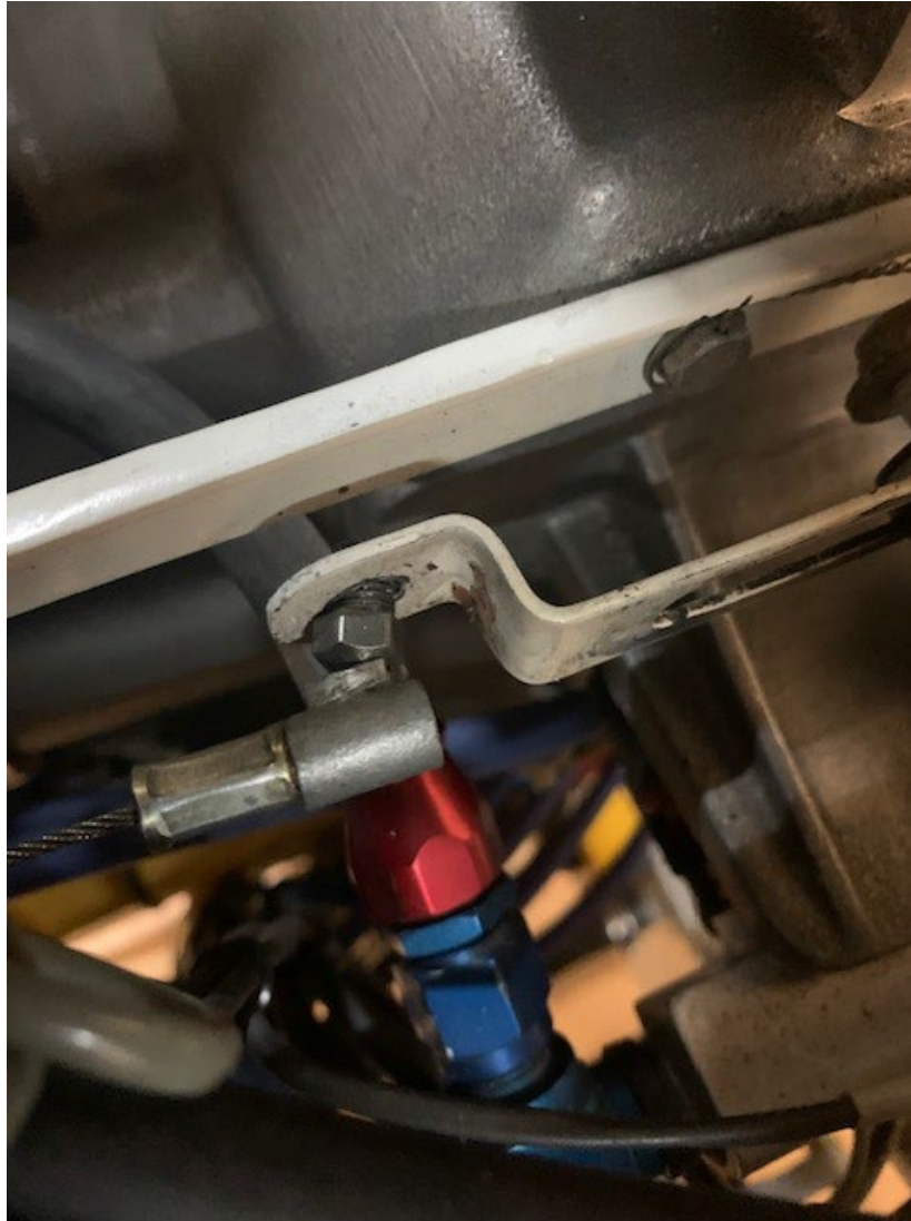
Photograph 3 - Throttle cable without securing nut (Courtesy of Owner)
