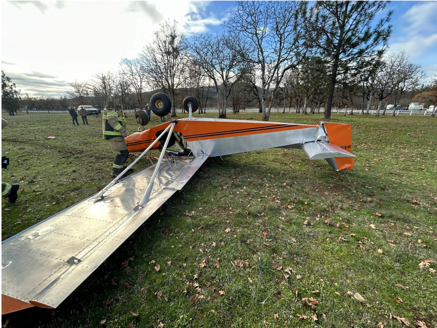
Photograph 2 - Empennage, wing and fuselage damage (Courtesy of Jackson County Sheriff)
