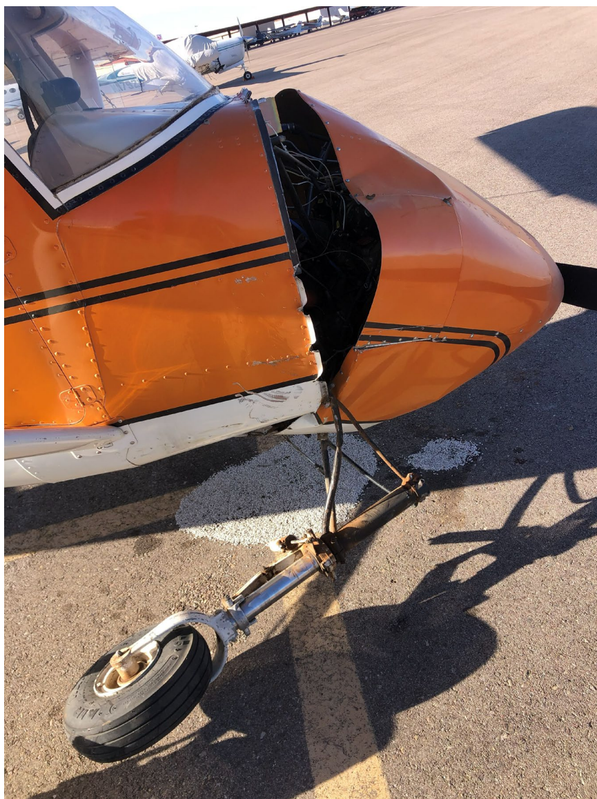
Photograph 2 - View of bent and severed engine mount attached to nose gear (Courtesy of Pilot)
