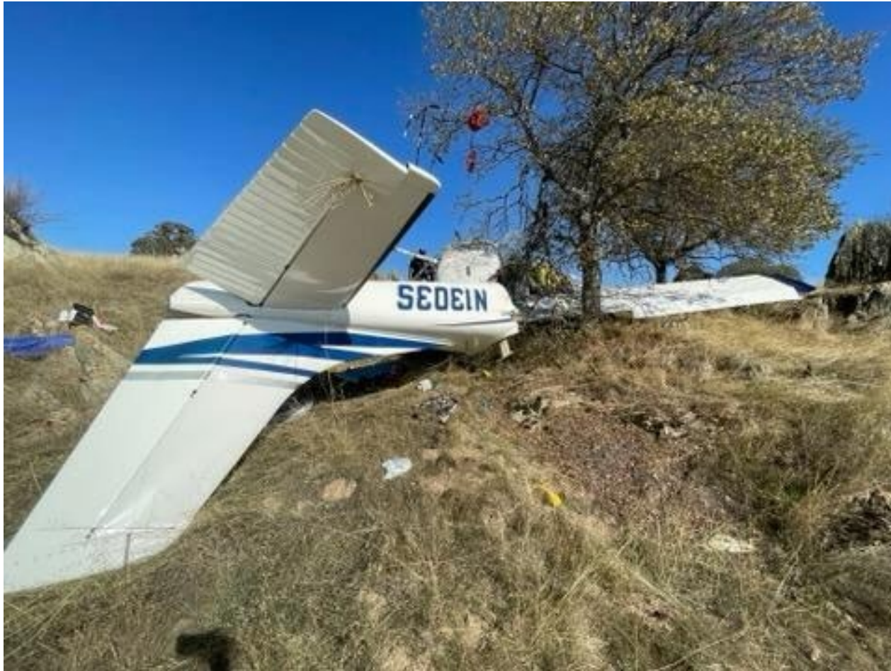
Photograph 2 - Empennage damage (Courtesy of Calaveras County Sheriff)
