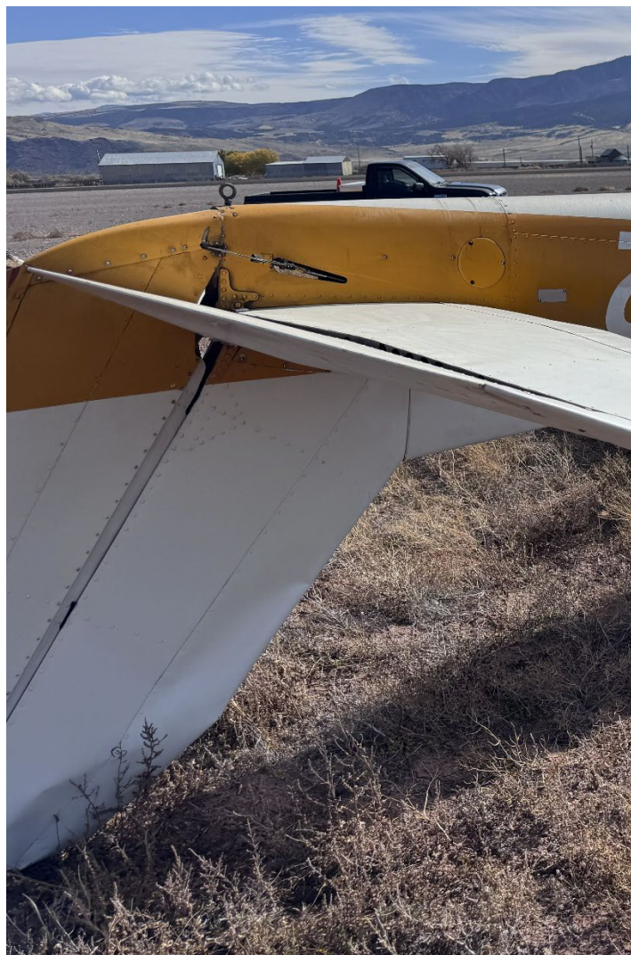
Photograph 1 - Vertical Stabilizer damage (Courtesy of Richfield PD))
