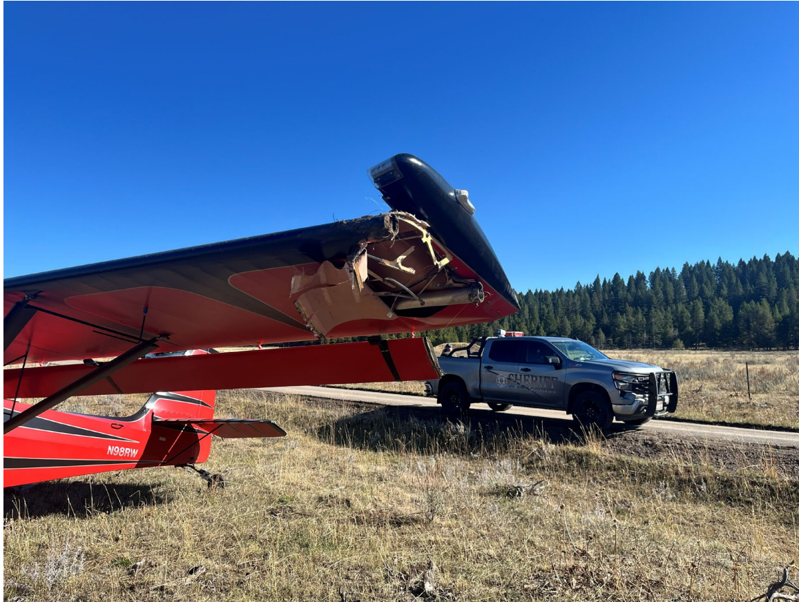
Photograph 2 - Front view of left-wing damage (Courtesy of Sheriff's Office)
