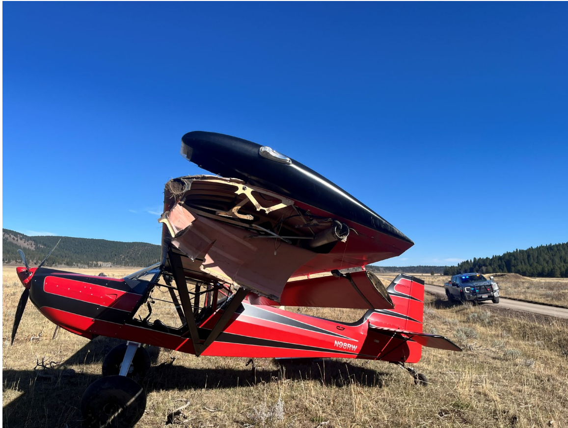
Photograph 1 - Side view of left-wing damage (Courtesy of Sheriff's Office)
