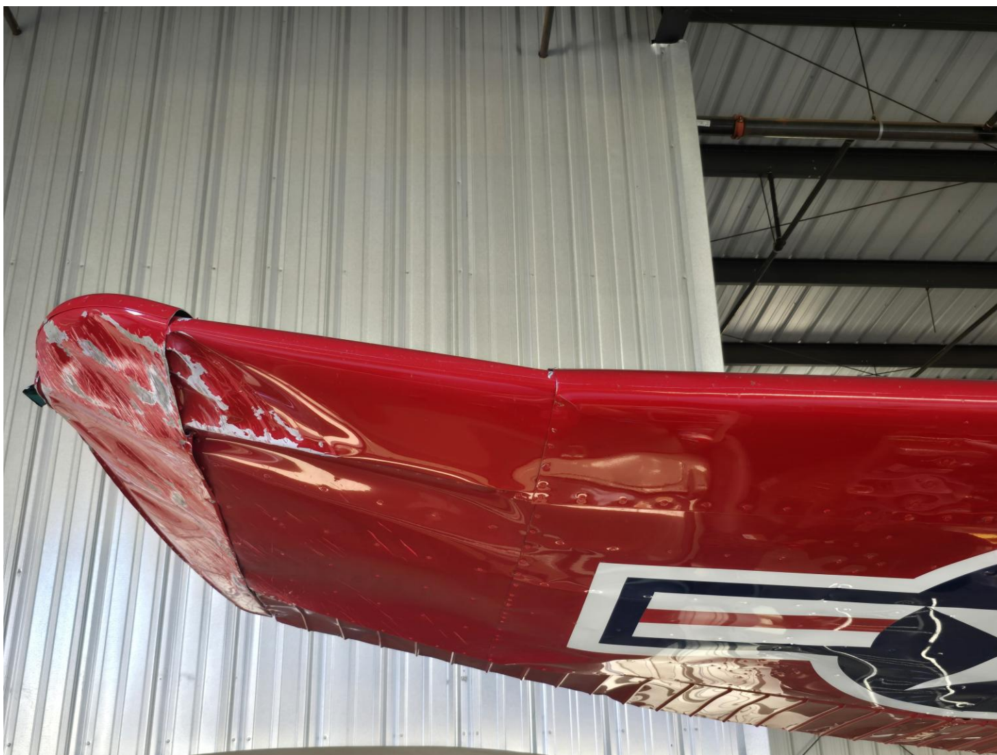
Photograph 1 - Right wing damage (Courtesy of pilot/owner)
