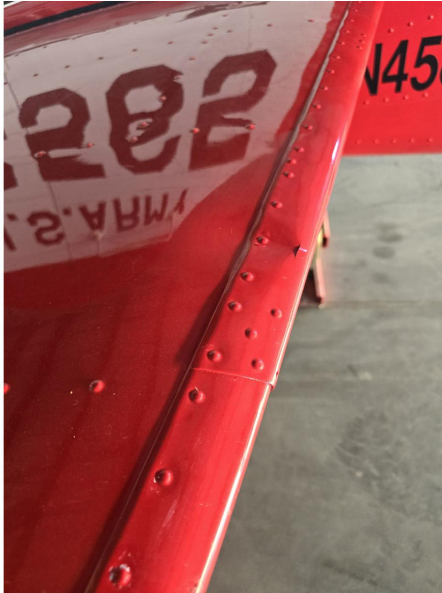
Photograph 2 - Empennage damage (Courtesy of pilot/owner)
