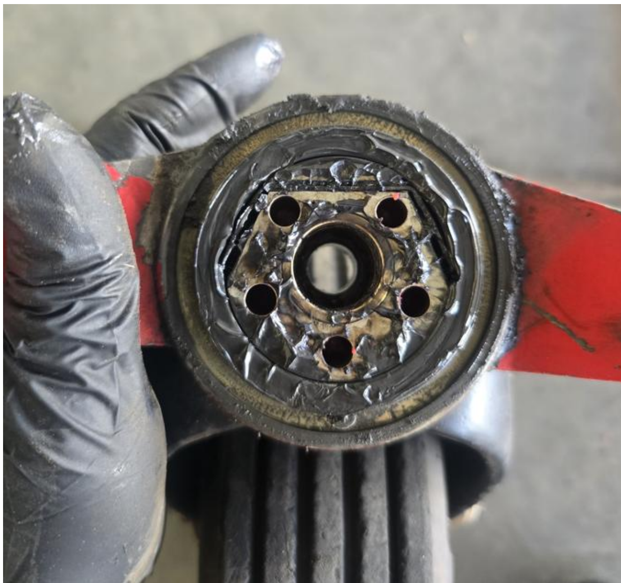
Photograph 8 - Tailwheel assembly internal, post-accident (Courtesy of pilot/owner)
