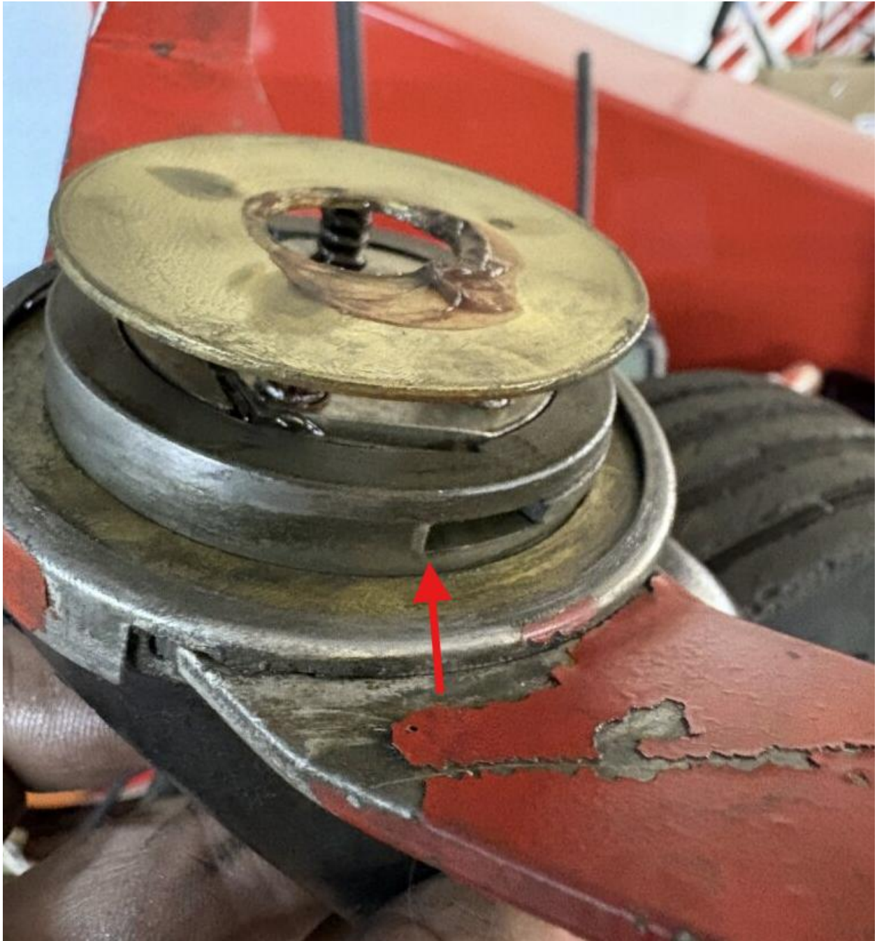
Photograph 12 – Steering arm assembly, outer race Arrow indicates outward material displacement along edge of pawl slot
