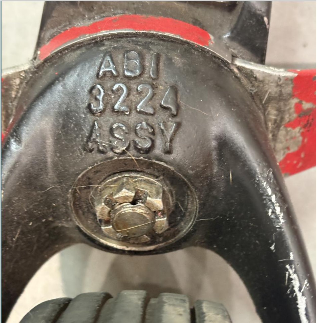
Photograph 2 – Tailwheel assembly, brand marking and part number
