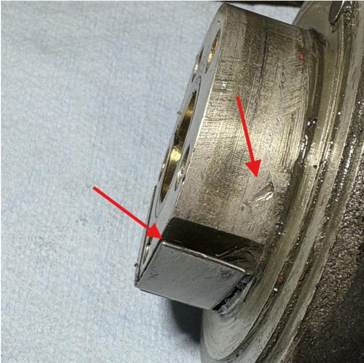
Photograph 5 – Tailwheel head, disassembled Arrows indicates gouges in outer bore, worn turn lock spring edges
