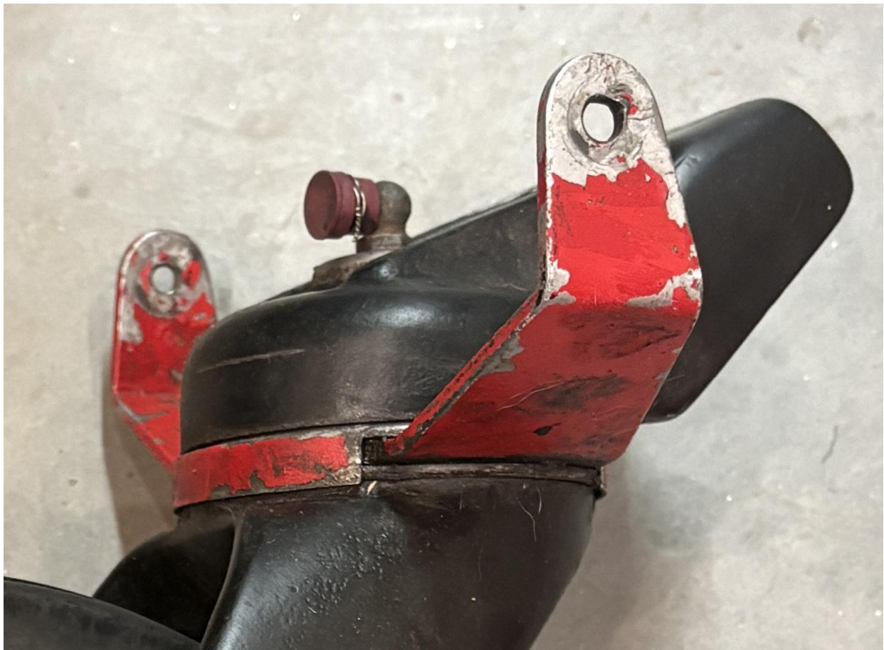
Photograph 1 – Tailwheel assembly, external, as received
