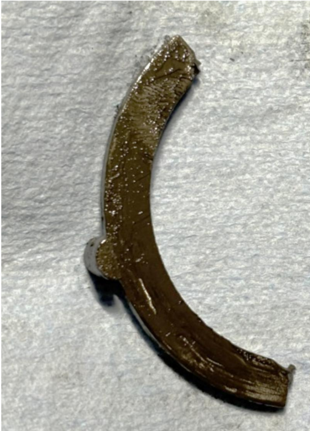
Photograph 8 – Tailwheel pawl, before grease removal
