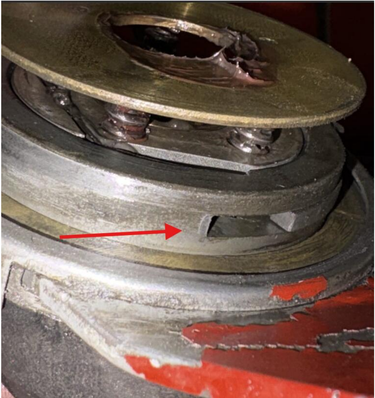
Photograph 11 – Steering arm assembly, outer race Arrow indicates outward material displacement along edge of pawl slot
