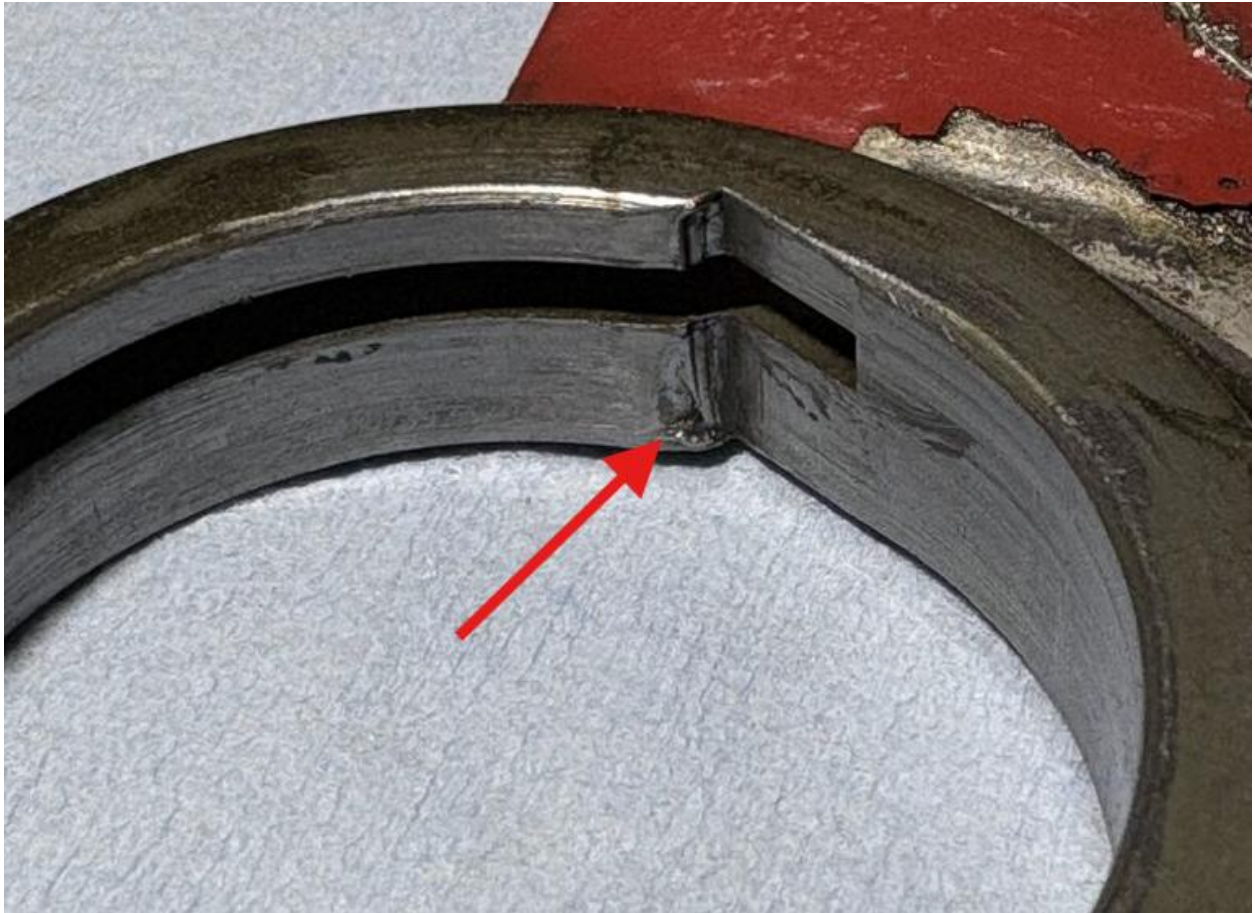
Photograph 6 – Tailwheel steering arm assembly Arrow indicates scratches/gouges at lock notch
