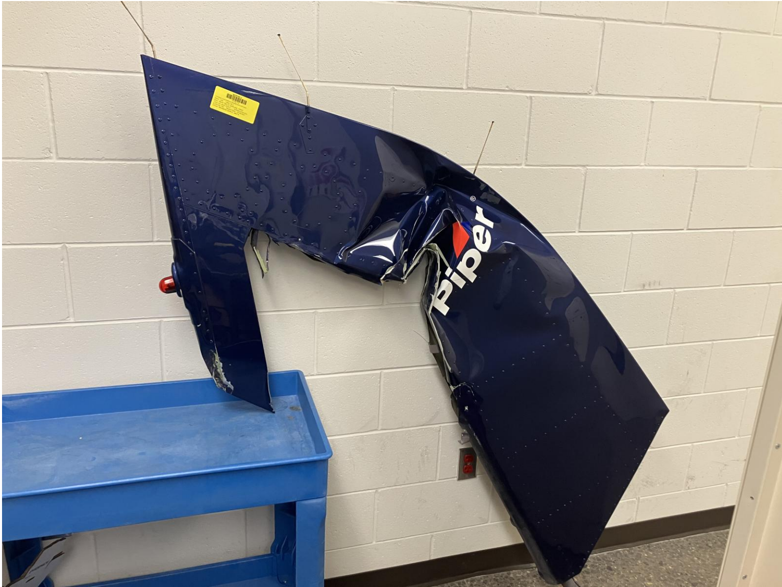
Photograph 2 - Rudder - Damage (Courtesy of FAA)
