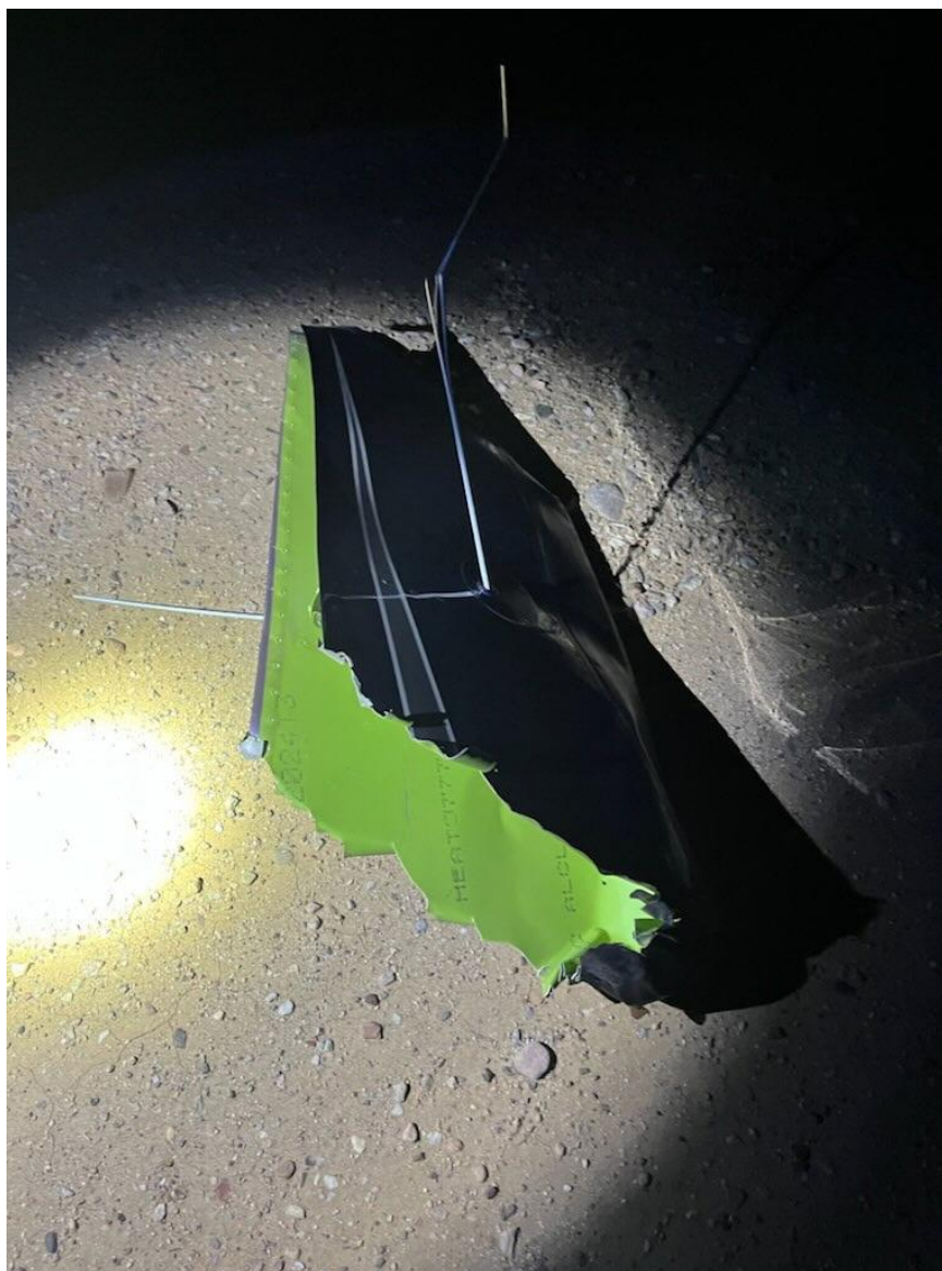
Photograph 4 - Vertical Stabilizer Damage On-Scene (Courtesy of FAA)
