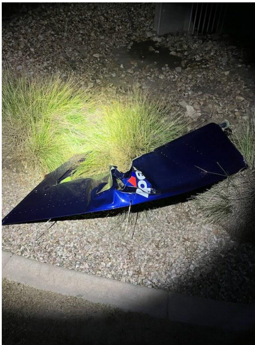
Photograph 5 - Rudder Damage On-Scene (Courtesy of FAA)
