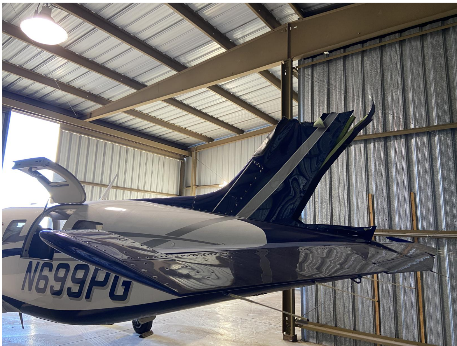
Photograph 1 - Airplane Empennage - Damage (Courtesy of FAA)
