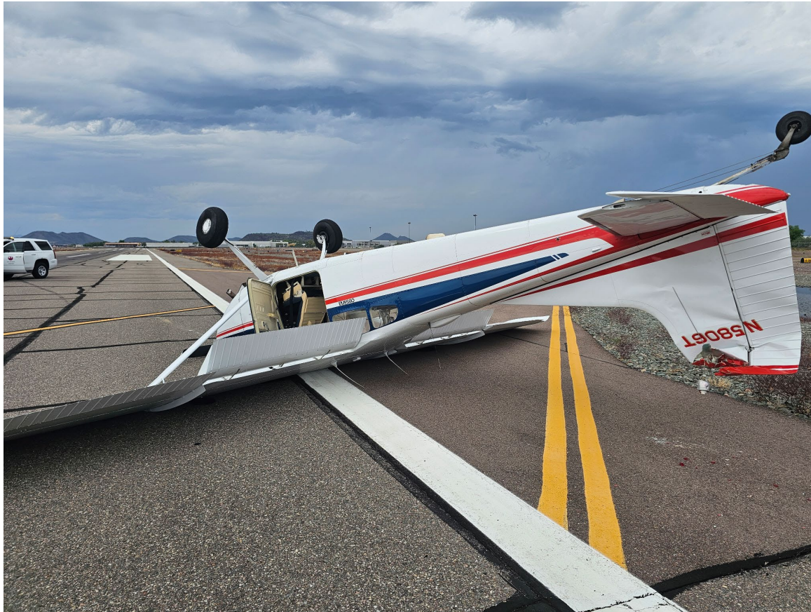
Photograph 2 - View of vertical stabilizer damage (Courtesy of Pilot)
