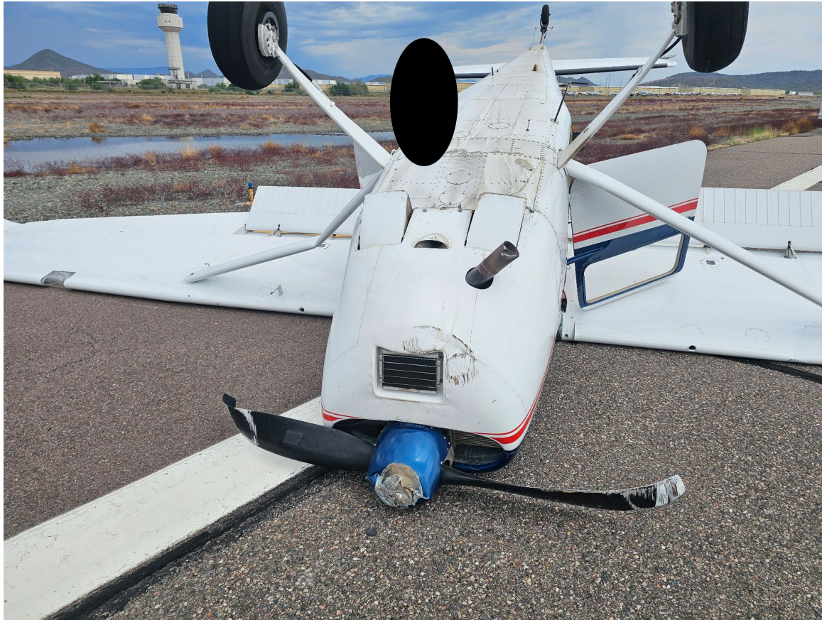
Photograph 1 - View of left-wing lift strut damage (Courtesy of Pilot)
