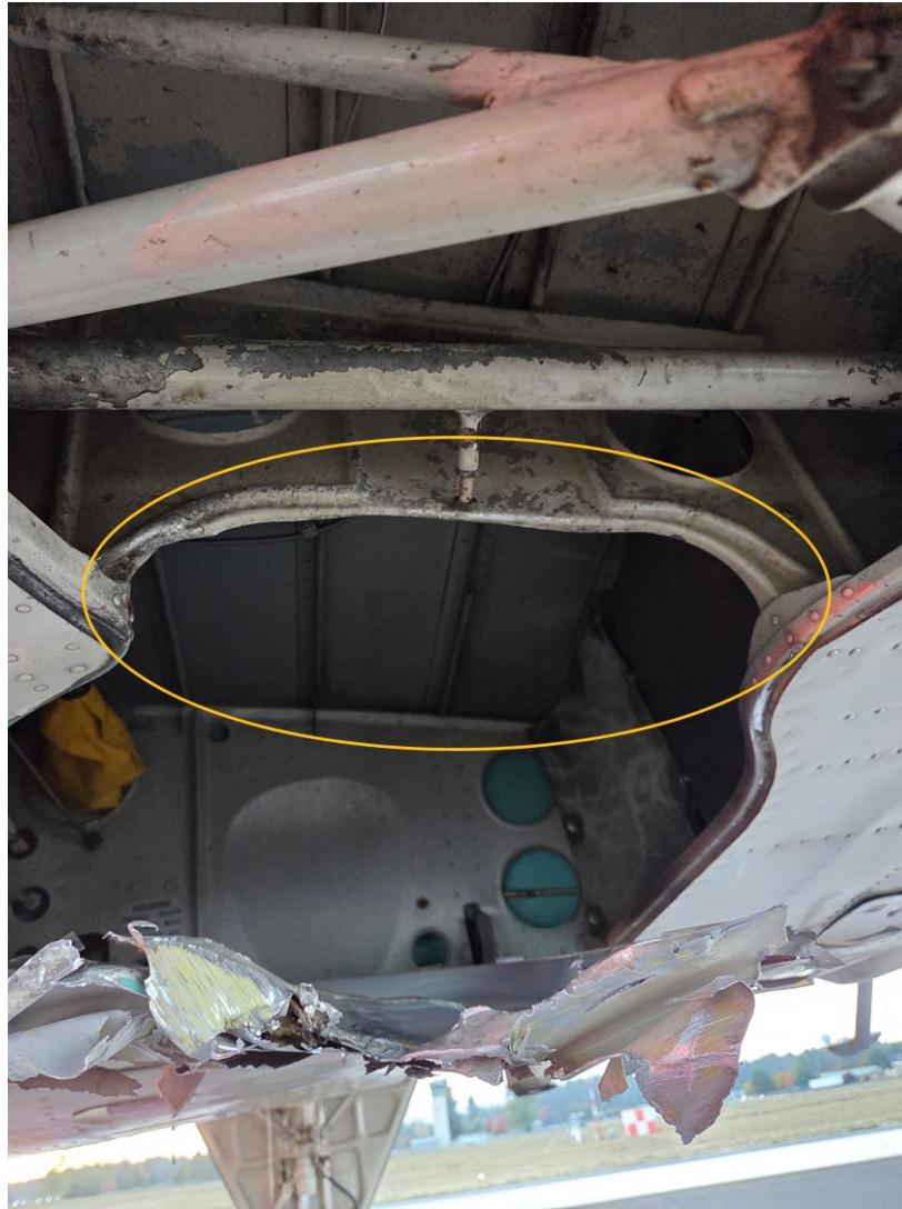
Photograph 2 - Left wing Rib damage (Courtesy of maintenance)
