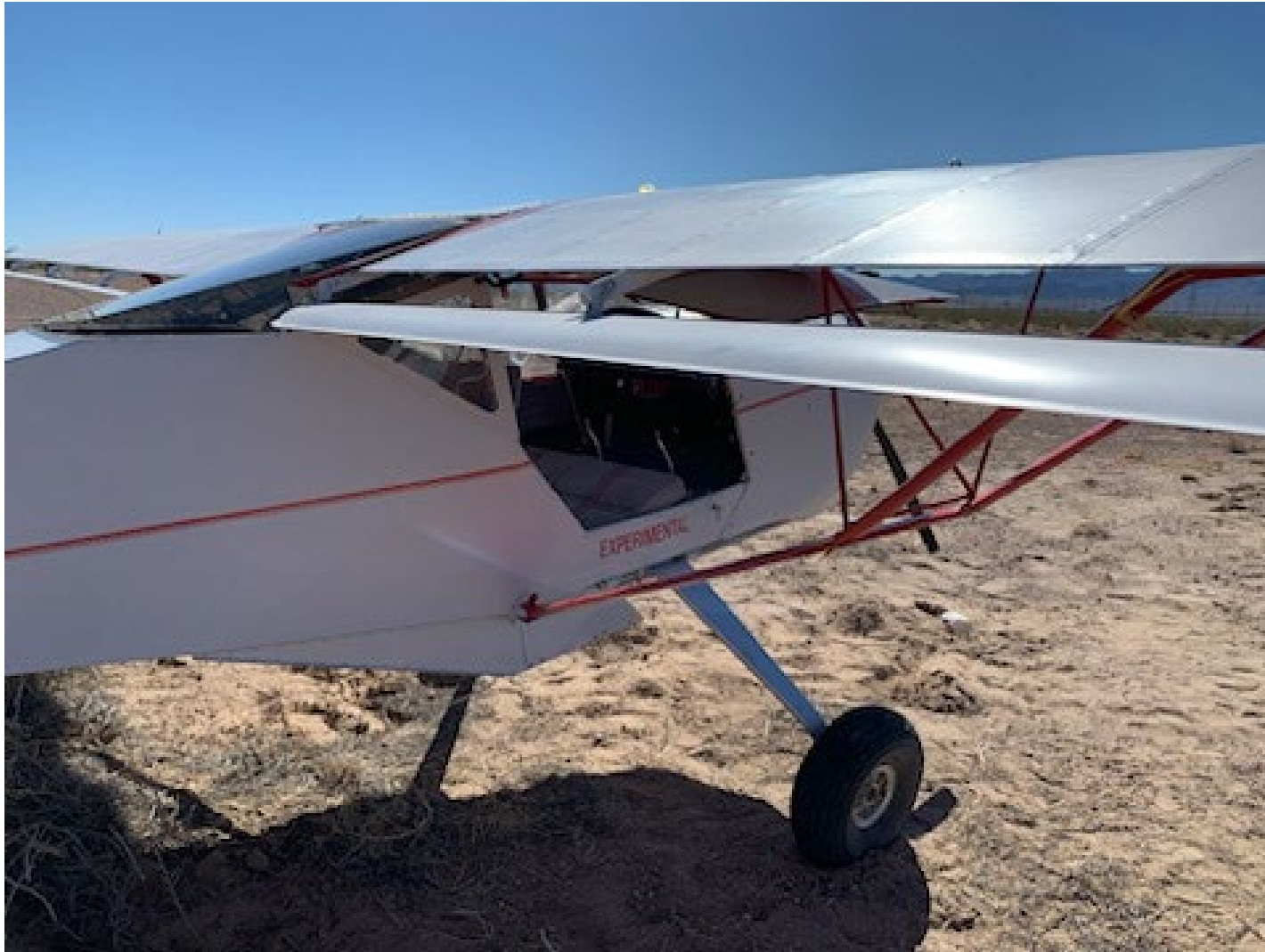
Photograph 2 - Right wing strut damage (Courtesy of Pilot)
