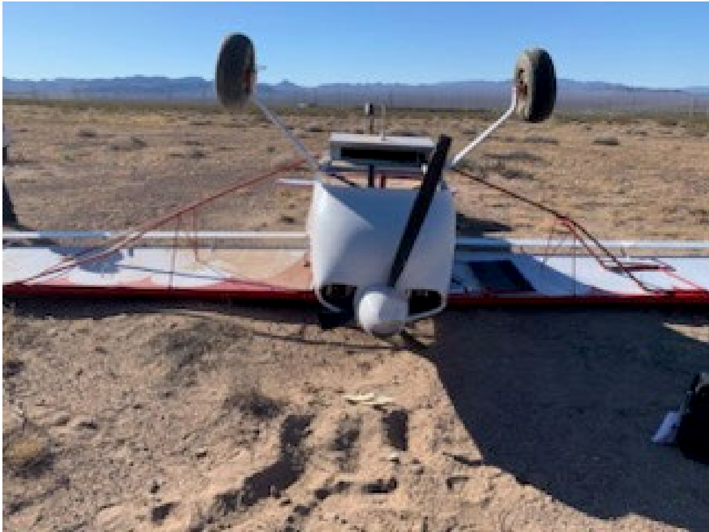
Photograph 1 - Right wing strut damage (Courtesy of Pilot)
