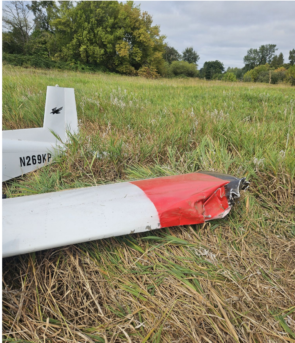
Photograph 2 - View of left-wing damage (Courtesy of Police Department)
